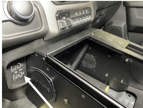
Position console up against lower center dash
