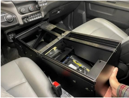
Carefully place console housing into vehicle on top of OEM center seat brackets.
