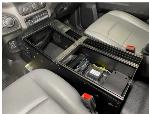
Console housing installed and ready to complete wiring, control head, and accessory installation. Slide P/N 25520 (1/4-20 hex nuts) (provided) into side extrusions as needed for side mounted accessories
