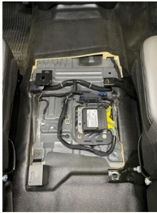
Remove center seat and front accessory pocket.
