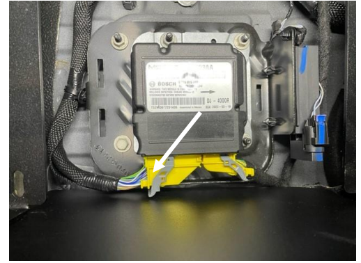
**Be careful not to damage OEM plugs and harnesses on transmission hump**
