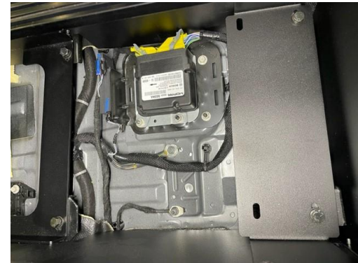
Attach console floor brackets to OEM seat mount points utilizing stock seat bolts
