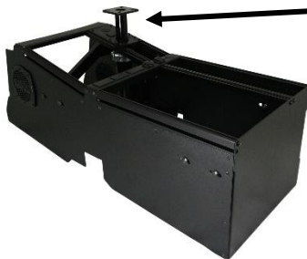
Optional C-HDM-214 pole can be installed at this time using the existing P/N 16223 (1/4" x 3/4" carriage bolts) in the side of console. Remove round knockout in pole face plate and attach plate to console around
