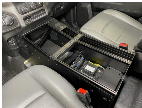
Console housing installed and ready to complete wiring, control head, and accessory installation. Slide P/N 25520 (1/4-20 hex nuts) (provided) into side extrusions as needed for side mounted accessories
