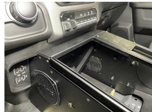
Position console up against lower center dash
