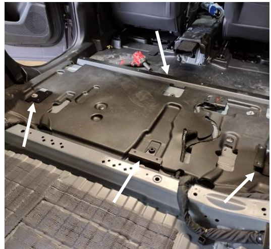
Install floor brackets.
