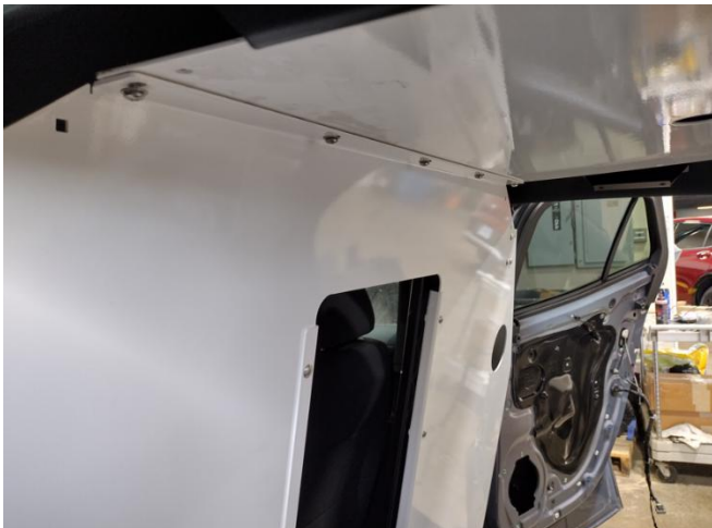
Install ceiling panel on top of front and rear bulkheads with 1/4" x 3/4" Phillips head bolts and flat washers. Install any remaining trim panels.
