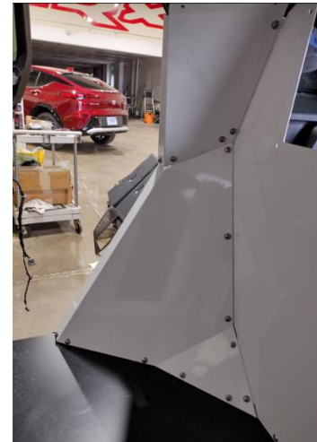
Install lower and mid pillar supports on both sides using 1/4" x 3/4" Phillips head bolts and flat washers.
