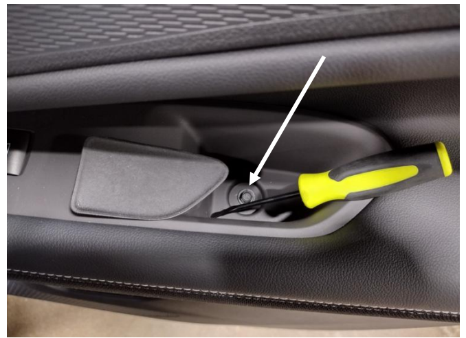
Remove plastic cover behind armrest handle. Remove screws.
