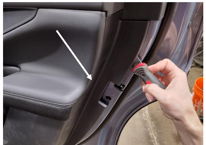
Remove / unsnap entire door panel from door. (Trim removal tool)
