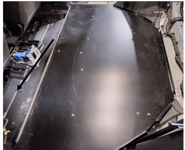
Install floor in vehicle. Attach floor to brackets with 1/4" x 3/4" Phillips head bolts and flat washers.
