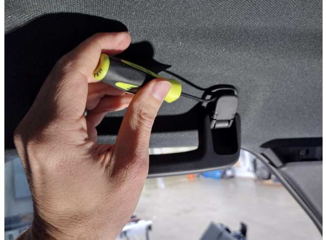
Remove the overhead grab handles.
