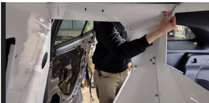
Install upper support and attach the handle bracket on each side.
