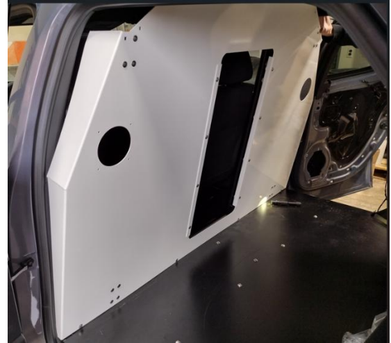
Install front bulkhead with 1/4" x 1/2" Carriage bolt and 1/4" Serrated nut.
