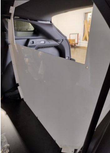
Install rear bulkhead with 1/4" x 1/2" Carriage bolt and 1/4" Serrated nut.
