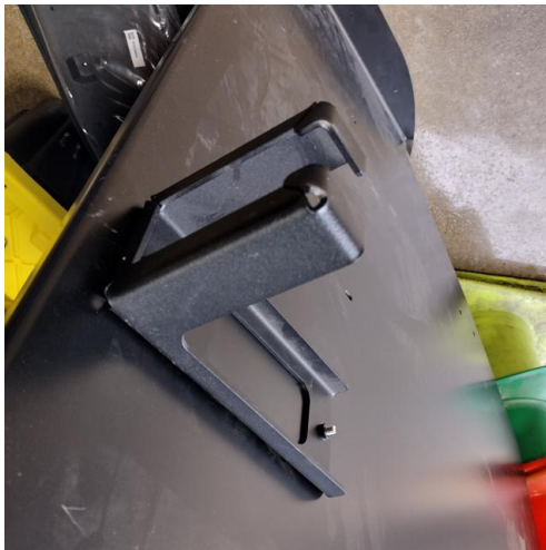
Install front floor support bracket to K9 floor with 1/4" x 3/4" Phillips head bolts and flat washers.
