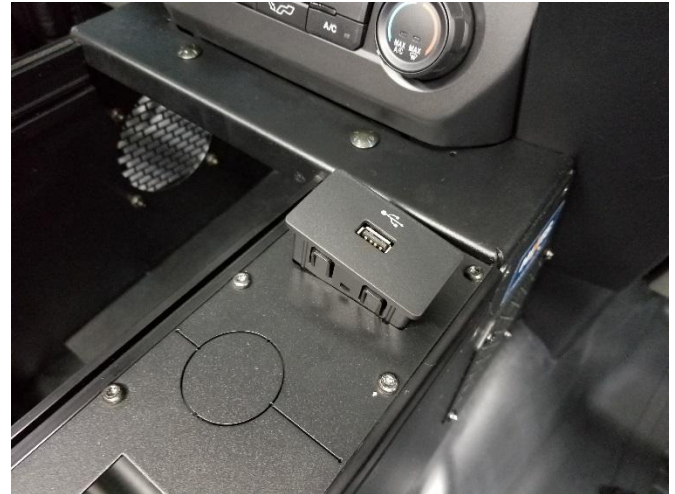
Install OEM AUX module into the console. Adaptor plate with #8 flat head screws provided for smaller Aux module. Blank plate provided if vehicle has no module for this location.
