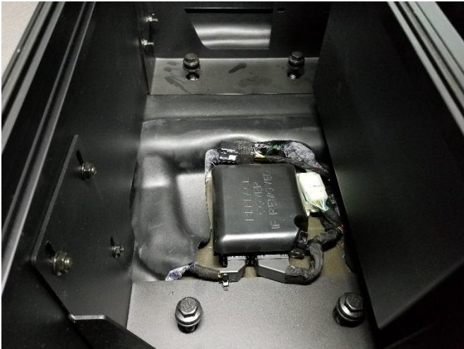
Loosely reinstall factory floor bolts through console floor brackets.
