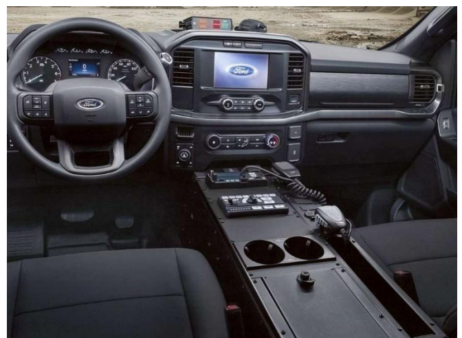
Console installation complete.
