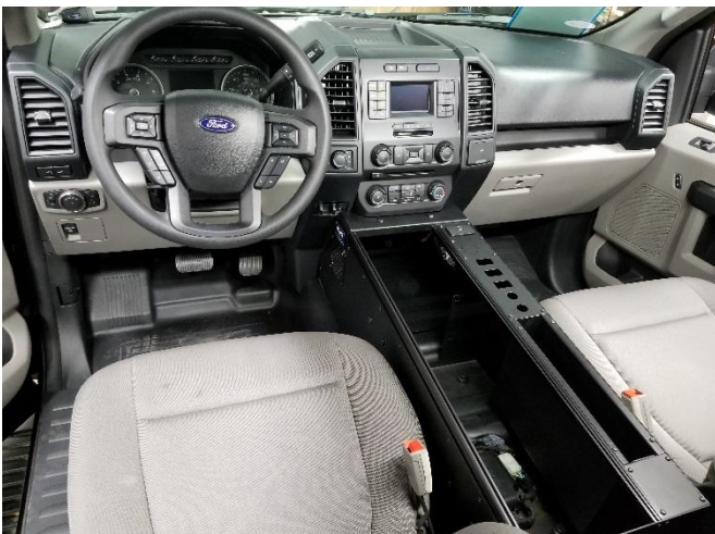
Install 1/4-20 hex nuts into side slots as desired for side mounted accessories. Install and wire equipment as desired.
