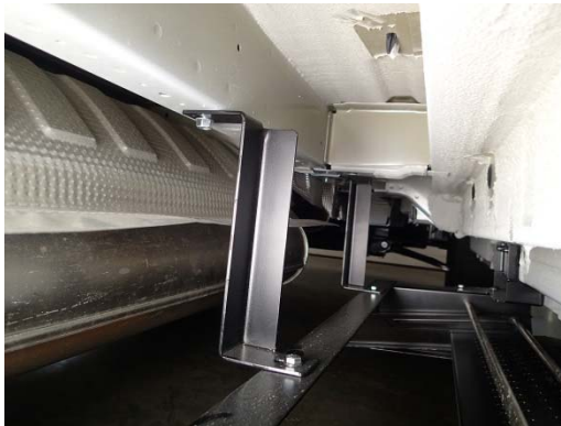
Attach the step assembly to the two rear frame supports (ST006578) using two (2) 5/16" x 1" bolts, four (4) washers, and two (2) 5/16" nylock nuts
