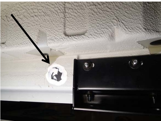
Insert the 1.5" grommet (GSM20017-2) into the hole and silicone around it to prevent rust.
