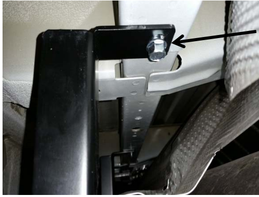
Line up the frame mounted support brackets (ST006578) with the unthreaded inserts in the frame. Use impact gun to drive the 3/8"x 1.75" thread cutting bolts into the inserts
