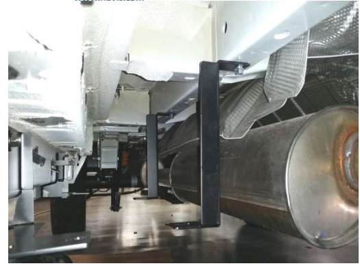
Repeat for the rearward frame support bracket
