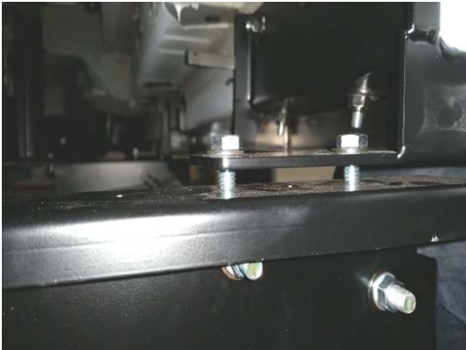
Loosely attach the step assembly to the body brackets using four (4) 5/16" x 1" bolts, eight (8) washers, and four (4) nylock nuts.
