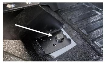
NOTE: Remove padding as necessary to allow supplied M10 bolt to pass through to OEM threaded hole. Repeat for both sides. Front brackets can sit on the padding.
