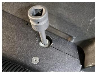
Loosely attach rear floor brackets to rear seat belt anchors on each side with OEM 12mm Torx bolts.
