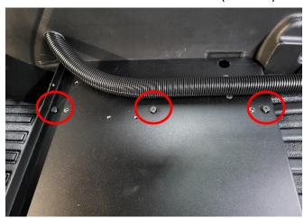
Loosely attach base plate to front floor brackets using supplied 1/4" x 1/2" Flat head bolts. (3 each side)
