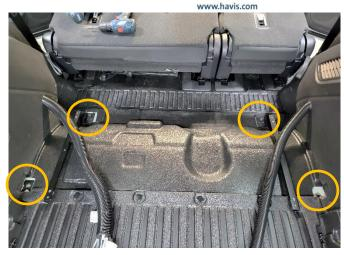
Determine 3<sup>rd</sup> row seat bolt locations in floor and loosely attach front floor brackets with supplied M10 bolts. Temporarily remove OEM M12 bolts from the rear seat belt anchor locations. (T50 Torx)
