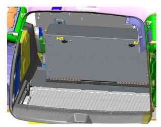
Attach C-SBX-101 to base plate using 1/4" x 1/2" bolts and washers included with box. Tighten all floor mount hardware. Installation complete.
