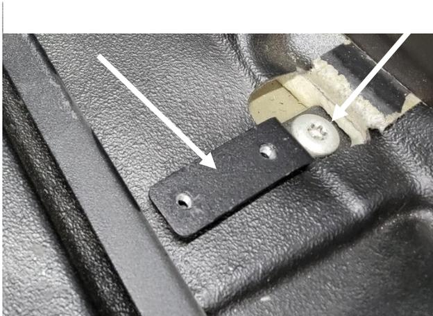
Locate OEM rear floor seat belt anchor bolts. Loosely attach rear floor brackets to OEM rear seat belt anchors on each side with existing OEM 12mm Torx bolts.
