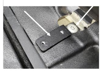
Locate OEM rear floor seat belt anchor bolts.
