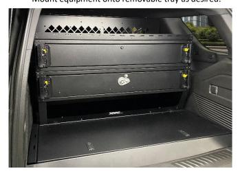
Attach main box lid with 1/4" x 5/8" Button head screws. Attach risers to main box with 5/16" Hex bolts and washers. Attach risers to drawer with 5/16" Thread-Forming Screws. Attach backing plate to risers and drawer with 1/4" and #10 Phillips hardware.
