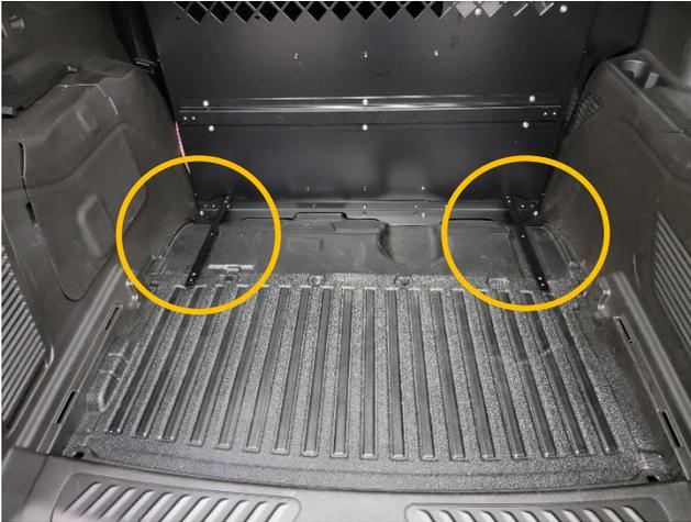
With K9-C26-XL or -PT installed, place driver and passenger side front floor brackets into vehicle.
