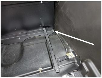
Attach each front floor bracket to 1/4 x 3/4 bolts in K9 rear closeout bracket. Also attach to pre-drilled holes with two (2) 1/4 x 3/4 self-threading screws. For K9-PT model, attach passenger side bracket with one (1) 1/4" x 3/4" Hex bolt and serrated nut.
