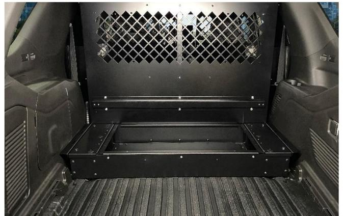
Place main box assembly onto brackets and attach with (10) 1/4" x 3/4" Hex bolts and star washers.
