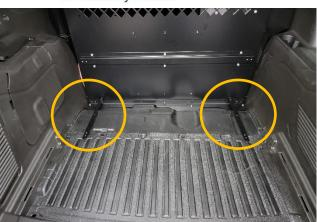
With K9-C26-XL or –PT installed, place driver and passenger side front floor brackets into vehicle.
