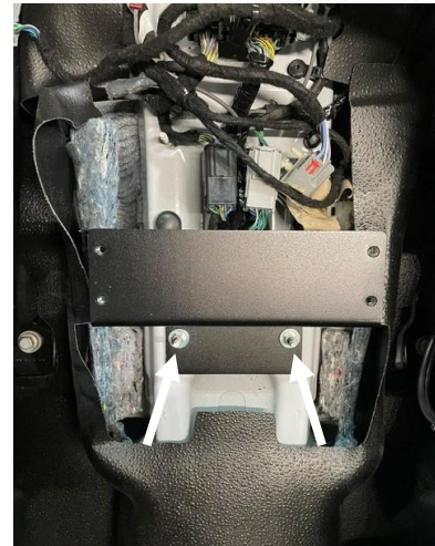
Attach rear mounting bracket to floor studs using previously removed OEM nuts. (10mm socket)
