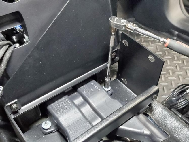
Retighten OEM ductwork nuts and bracket hardware.
