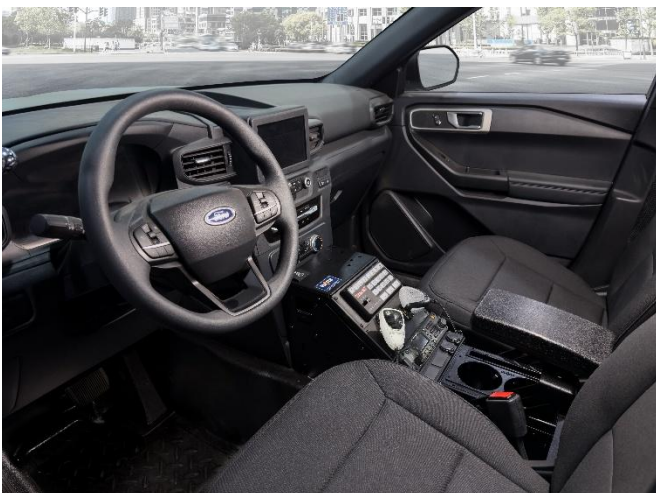
Place console over previously installed brackets attach with carriage bolts, serrated nuts, 1/4-20 X 3/4" screw hex head cap and 1/4" washer. Ensure console is tight to dash. Tighten all hardware.
