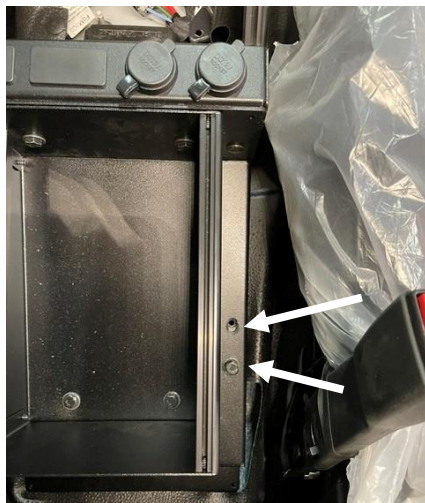
Place console over previously installed brackets attach with carriage bolts, serrated nuts, 1/4-20 X 3/4" screw hex head cap and 1/4" washer. Ensure console is tight to dash. Tighten all hardware.
