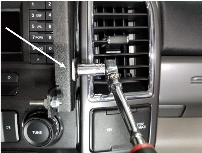
Line up the lower frame to the side support bracket and attach with 1/4" bolt, flat washer and serrated nut.
