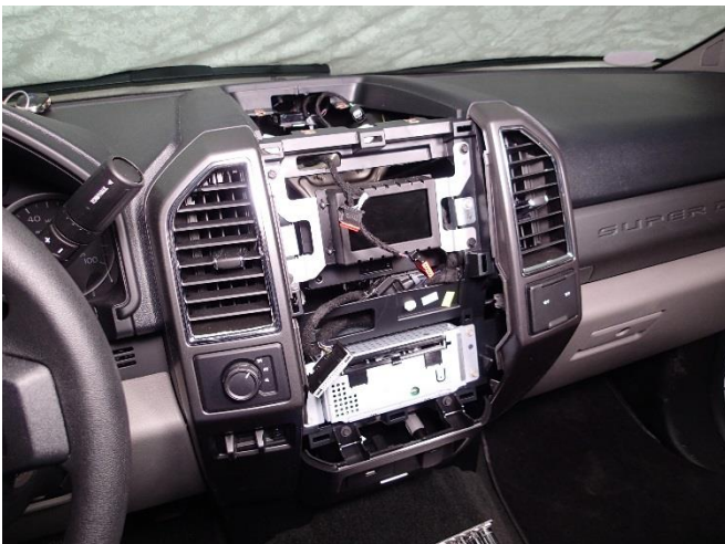
Carefully remove center HVAC and radio control trim bezel.
