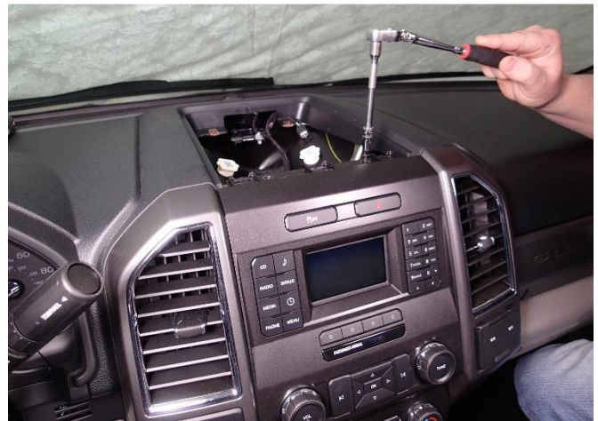
Remove two (2) fasteners from upper display area. (7mm socket)
