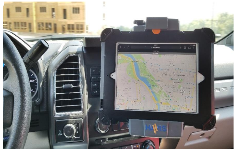
Run wire harness and test computer. Installation is now complete.
