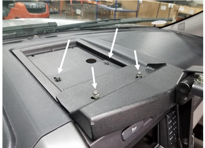
Place main hinge frame on top and loosely attach to tray with 10-32 x 1/2" machine screws and flat washers. Attach to OEM speed nuts with #10 sheet metal screws and flat washers.
