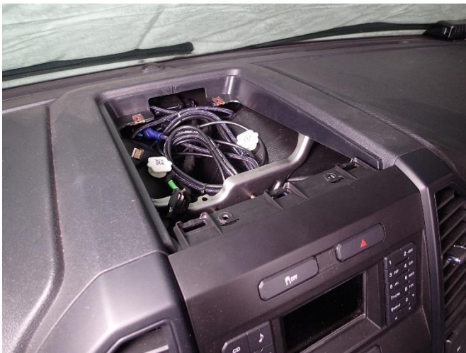
Lift up and remove OEM plastic tray. This tray will not be reused.
