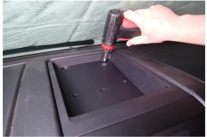
Remove two (2) fasteners from the forward section of the tray. (7mm socket)
