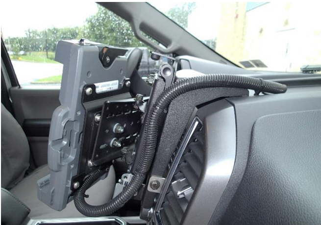
Determine desired position for your specific computer and attach to DMM swivel plate using 1/4"x 3/4" carriage bolts, PVC spacer, nylon washers, steel washers, and nylock nuts. Tighten so that the dock rotates smoothly.
