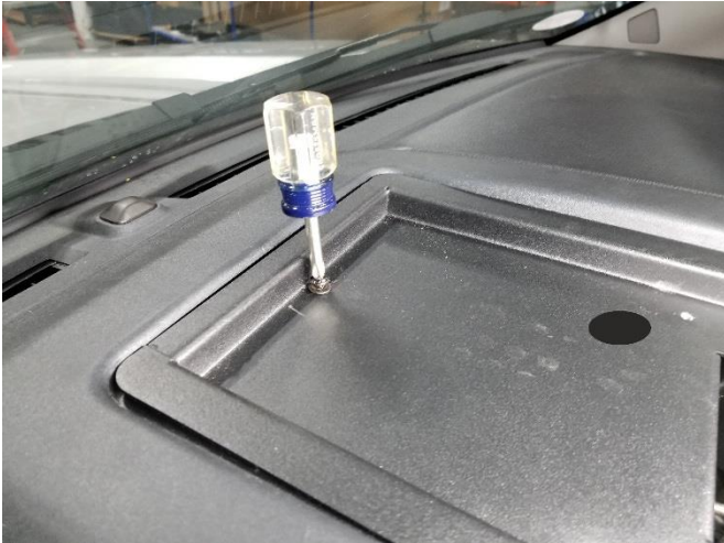
Attach forward end of tray with 10-32 x 1/2" machine screw and #10 flat washer.
