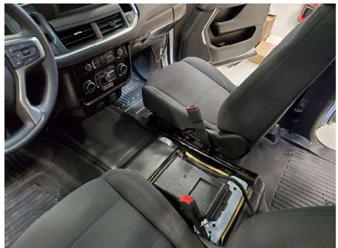
**We highly recommend bolting seats back in after console is installed. This makes installation much easier.**
