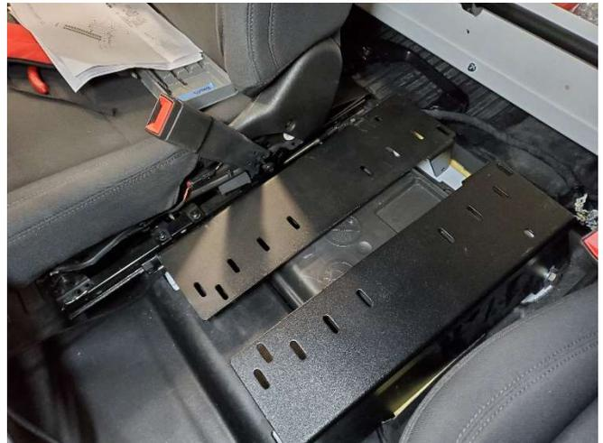
Level driver and passenger side brackets and loosely attach floor mount hardware.
