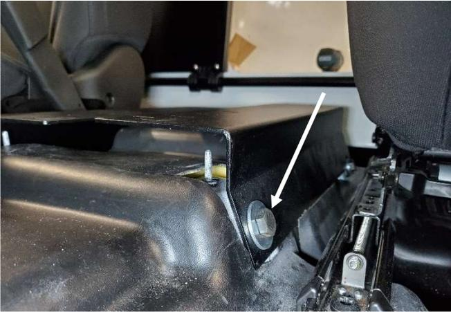
Place floor, mounting brackets over holes in floor and attach using M12 x 1.75 bolts and 7/16" flat washers.
