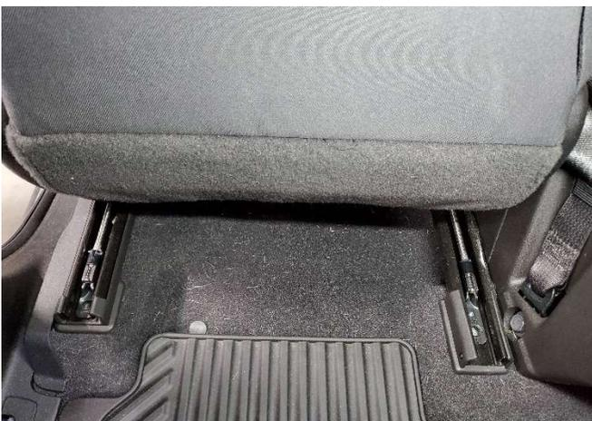
To remove bolts, the seat will need to be unbolted and shifted out of the way.
