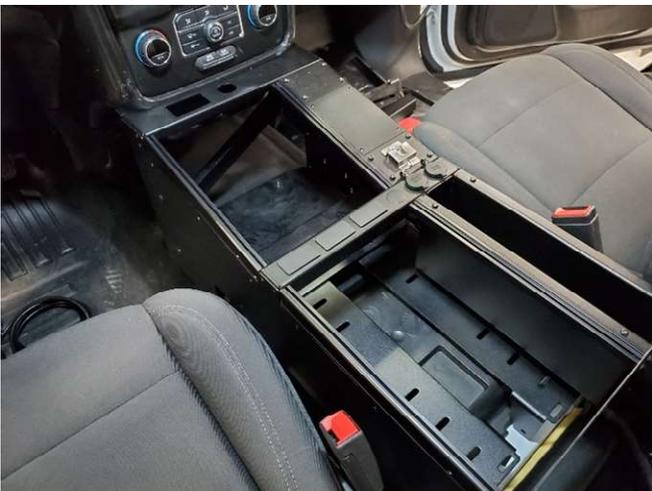
Place console housing with forward support bracket onto floor mounting brackets and slide housing toward dash.
