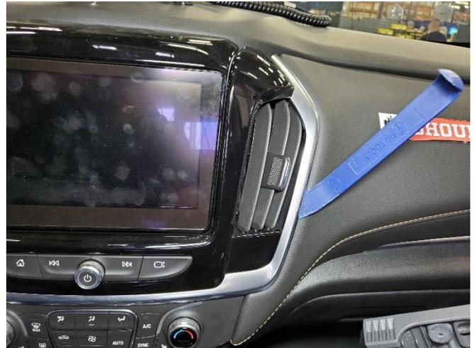
Carefully pry along sides of trim with a panel removal tool.
