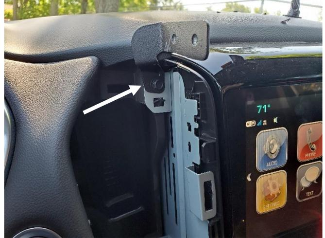
Remove OEM fastener and attach driver side upper mounting bracket.
