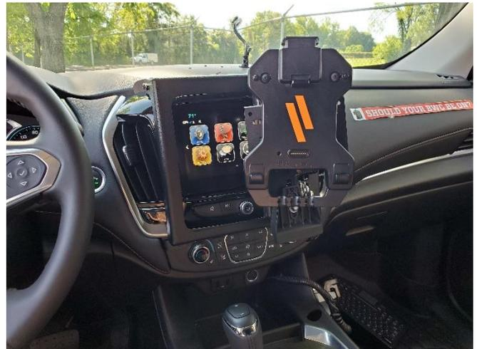
Confirm correct placement of dock and make sure rotation movement is smooth and latching works correctly.
