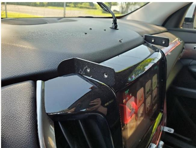
**Note:** Carefully snap trim back in making sure not to scratch against upper mounting brackets.
