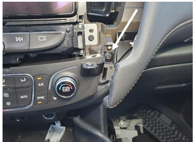
Remove OEM fastener and attach passenger side lower mounting bracket.
