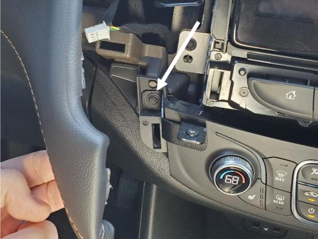
Remove OEM fastener and attach driver side lower mounting bracket.
