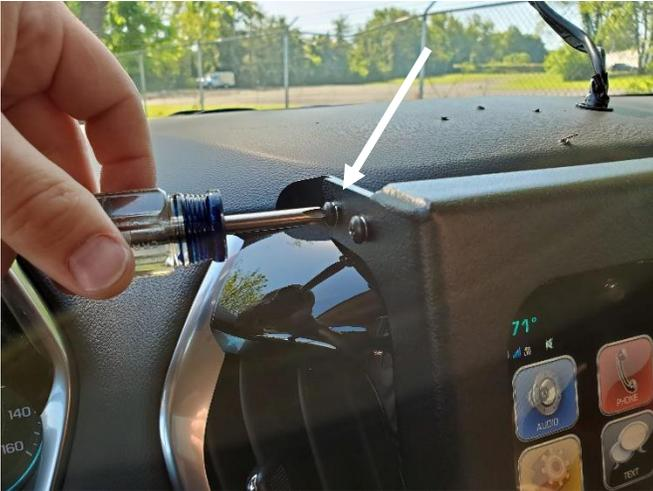
Place DMM frame onto mounting brackets and attach using 10-32 x 3/8" machine screw and flat washer.
