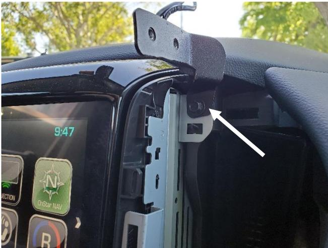
Remove OEM fastener and attach passenger side upper mounting bracket.
