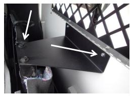
Attach the upper rear support bracket to existing rear wall hinge studs and to OEM threaded holes with previously removed seatbelt hardware.
