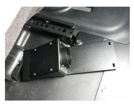
Slide vent adaptor over factory blower vent under seat.
