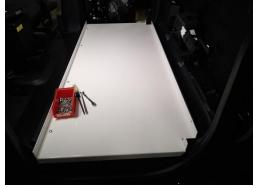
Attach floor to the front base mounting bracket using four (4) 1/4" x 3/4" carriage bolts and serrated nuts.
