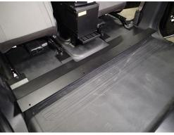
Install the front mounting bracket lining up to the holes for the seat bolts. Re-install previously removed seat bolts and tighten.
