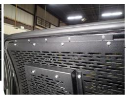
With upper mount bracket attached to window guard, mark mounting hole locations on upper door / window frame. Drill 5/32" holes and attach with # 10 x 1/2" flat head sheet metal screws.
