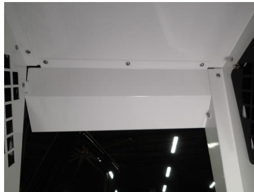
Loosely attach upper filler panel with 1/4 x 3/4 Phillips pan head bolts and washers. Install one (1) carriage bolt and nut to front wall Repeat process for driver's side
