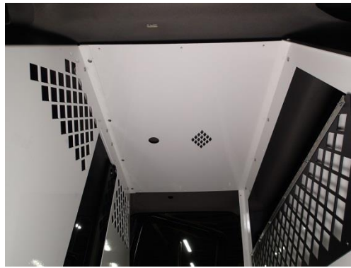
Attach the ceiling to the front and rear walls with 1/4" x 3/4" carriage bolts and nuts.
