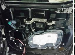
Disconnect door latch cable and lock pin. Remove speaker. (7mm socket) Remove window switch from door panel and set aside.
