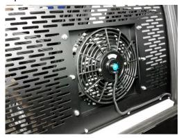
Attach optional 10" fan and fan mount to window guard with 1/4" hardware and spacers as per the instructions provided in the K9-A-104 kit.
