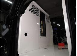
Attach front wall to "B" pillar brackets and floor using 1/4" x 3/4" carriage bolts and serrated nuts.
