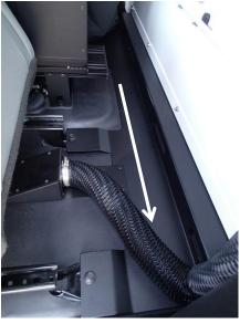
Secure the vent hose to the bottom corner of the floor bracket using supplied 15" wire tie.
