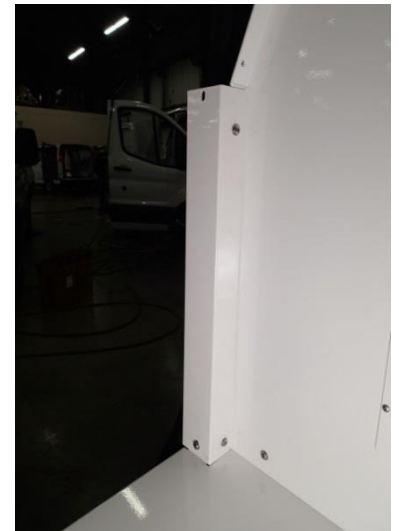
Loosely attach side filler panel to rear wall with 1/4 x 3/4 Phillips pan head bolts and washers.
