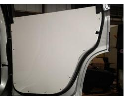
Hook door panel on the weather stripping and centering it on the door. Attach panel with # 10 x 1/2" Phillips pan head sheet metal screws.
