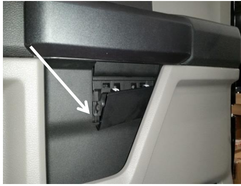
Remove two (2) bolts behind access cover in middle of door panel. (10mm socket)
