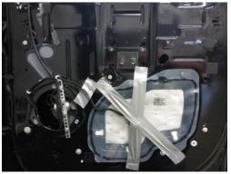
The window switch must remain plugged in proper operation. Taping the switch to the interior side of vapor barrier or wrapping in plastic bag is recommended to avoid problems with moisture.
