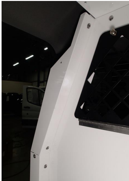
Loosely attach upper side filler panel to rear wall with 1/4 x 3/4 Phillips pan head bolts and washers.
