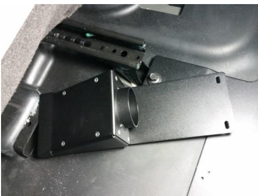
Slide vent adaptor over factory blower vent under seat. One each side.
