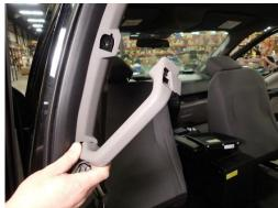
Remove the factory grab handles by gently prying off bolt covers. Remove two (2) M6 bolts (7mm socket)
