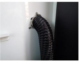
Attach supplied vent hose to vent adaptor and round vent with supplied hose clamp. Hose needs to be cut into two (2) 3 foot pieces.
