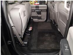
Note: Seat belts must be plugged back into OEM harness (to original plug location). Wire tie seat belts in out of the way location prior to K9 floor being installed.
