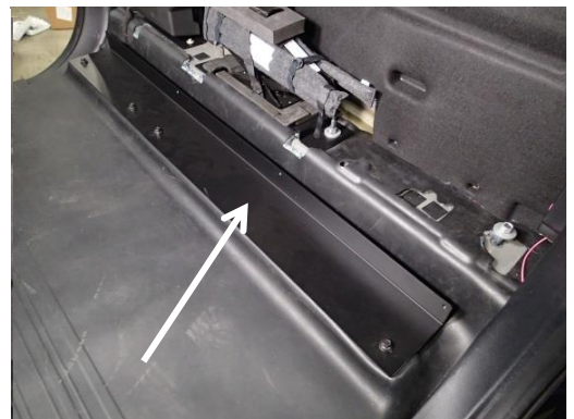
Install the rear mounting bracket with the flange towards the rear. Use previously removed seat bolts.
