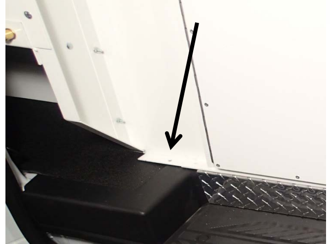
On the three compartment insert the side through bolt will not be used. This is due to obstructions under the van.
