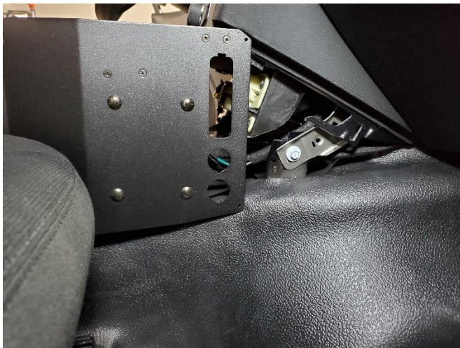
With the front printer trim panel installed, place the console tight to the dash. It is easiest to pick up the rear of the console and slide it towards the dash and then lower the rear.
