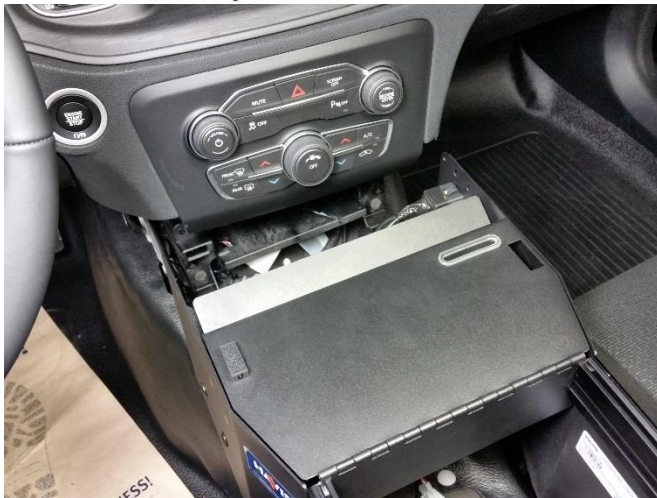
Slide console up to the dash leaving space for the next step.
