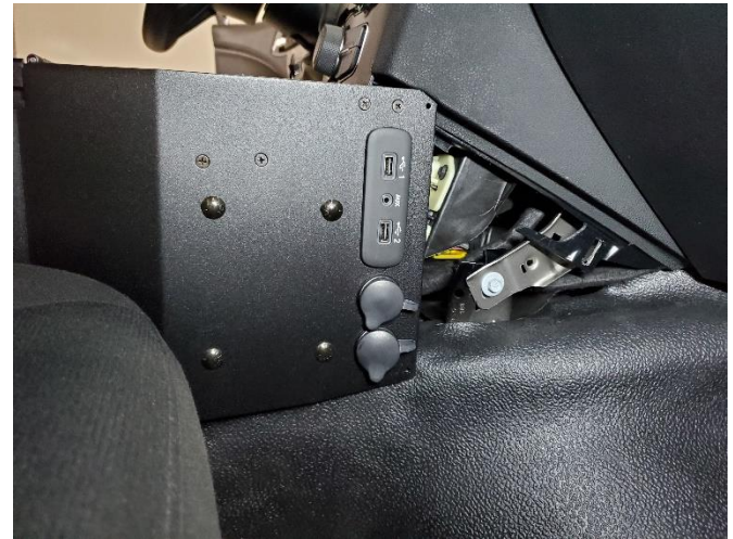
Install OEM AUX panel and 12V outlets into the side of the console. Plug into factory harnesses.
