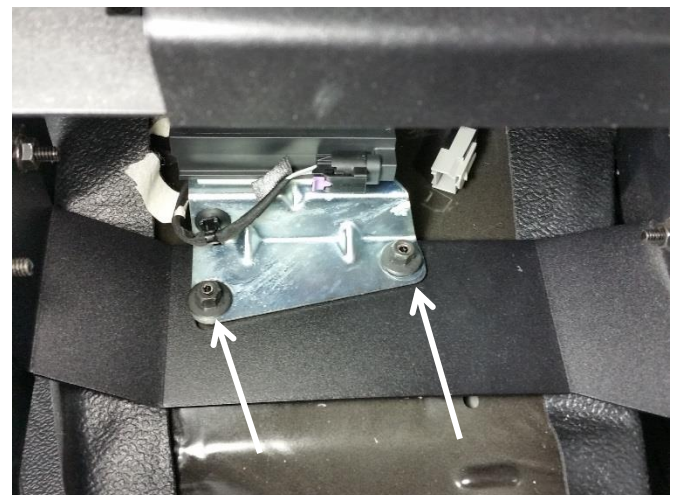
Place the ignition key sense module on the OEM studs and reinstall previously removed nuts.
