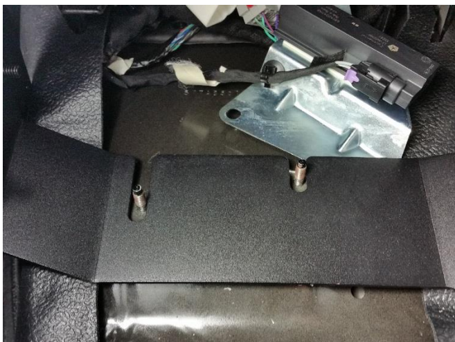
Make sure the ignition key sense module is moved out of the way and line up the U bracket to the OEM studs.
