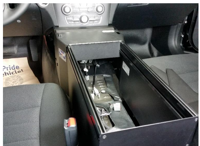
Place console housing into vehicle.
