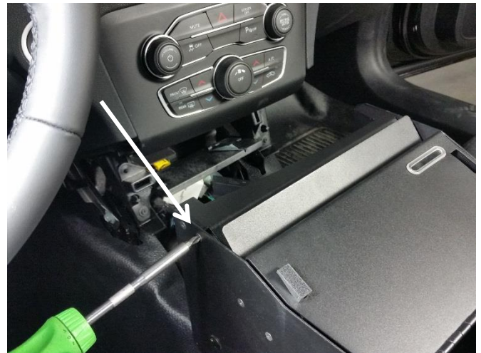
Attach the front printer trim panel (12593) using four (4) #8-18 x 1/4" flat head screws. (16425)
