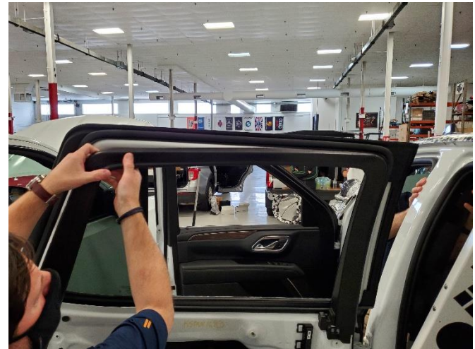
Gently remove trim around window frame.
