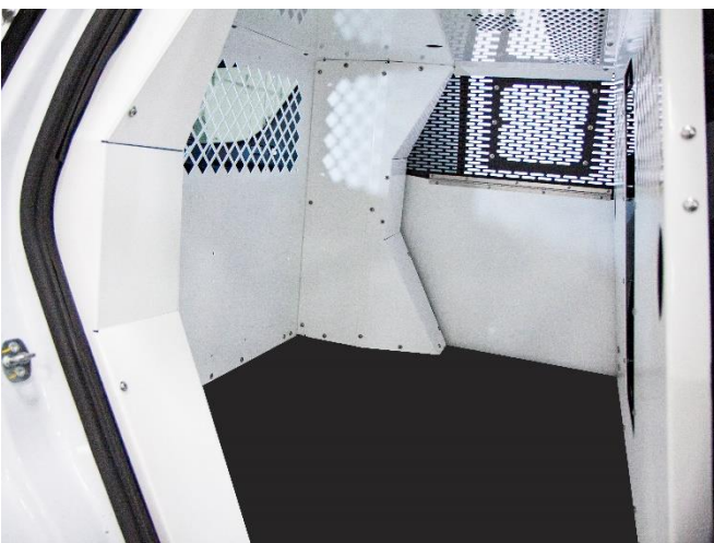
Place rubber mat into kit after silicone is dry.
