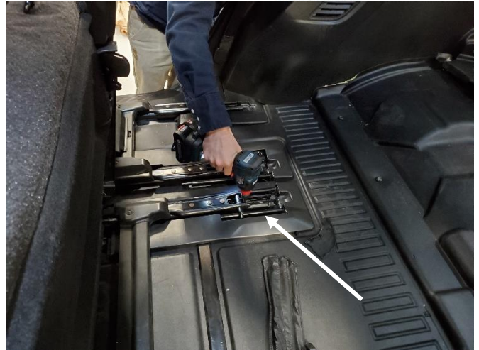
Flip seat seats forward to access hardware.
