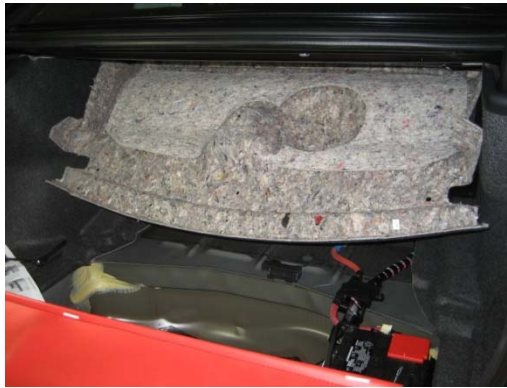
Remove upper trunk liner if desired. It is not necessary to completely remove, but it may make bracket installation easier.
