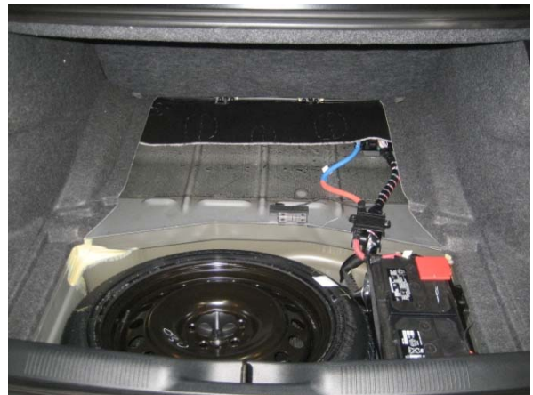
Remove carpeted floor liner for bracket installation. Remove upper trunk liner if desired.
