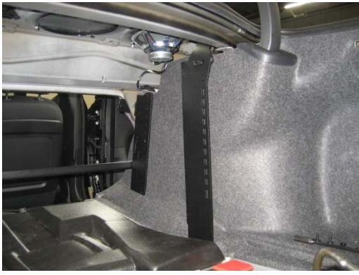
Passenger side brackets in place.
