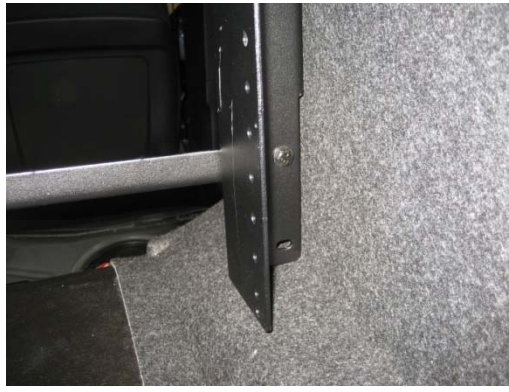
Forward bracket is positioned slightly above trunk liner.
