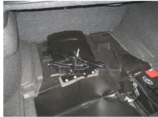
Remove spare tire/jack hold down bracket (15mm, 13mm, 18mm)
