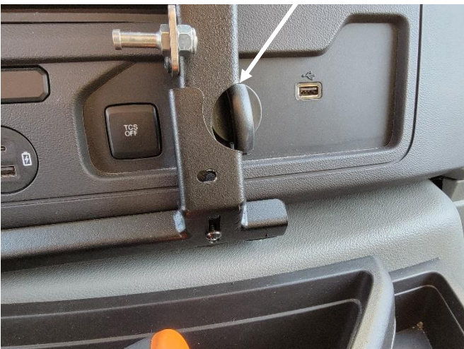
Line up holes allowing clearance for 12-volt socket.
