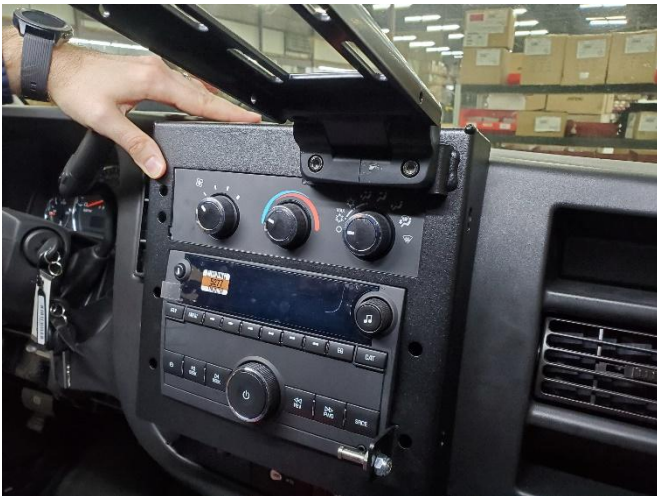
Tighten radio and HVAC controller through access holes in front of frame. Cover holes with 3/8" dome plugs supplied with kit.
