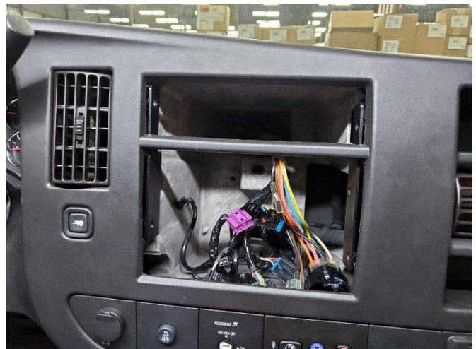
Reinstall previously removed dash.
