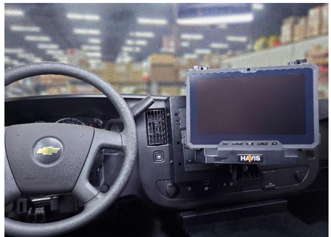
Route wiring as needed along the side of the DMM frame using wire tie holes. Test up / down and side to side motion to confirm wires have adequate slack and strain relief. Installation is now complete
