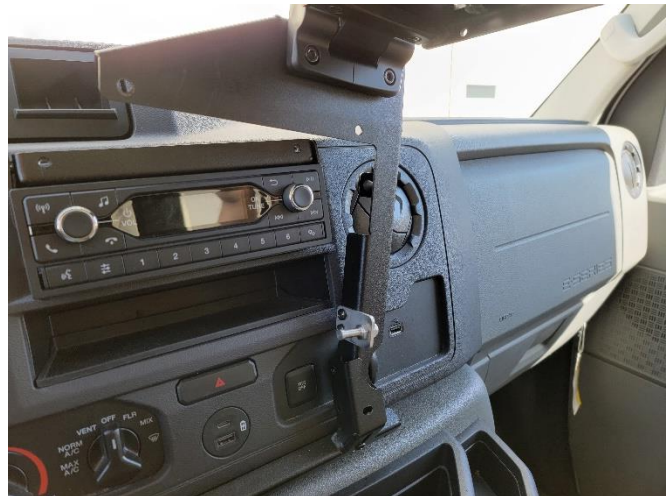
Place upper frame assembly onto lower frame.
