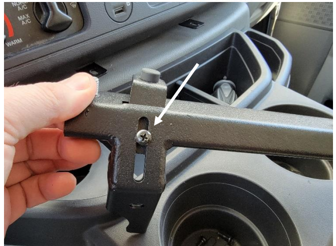
Slide lower radio, mounting bracket foot into lower frame assembly.
