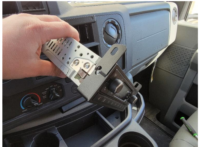
Slide up until snug on radio chassis.
