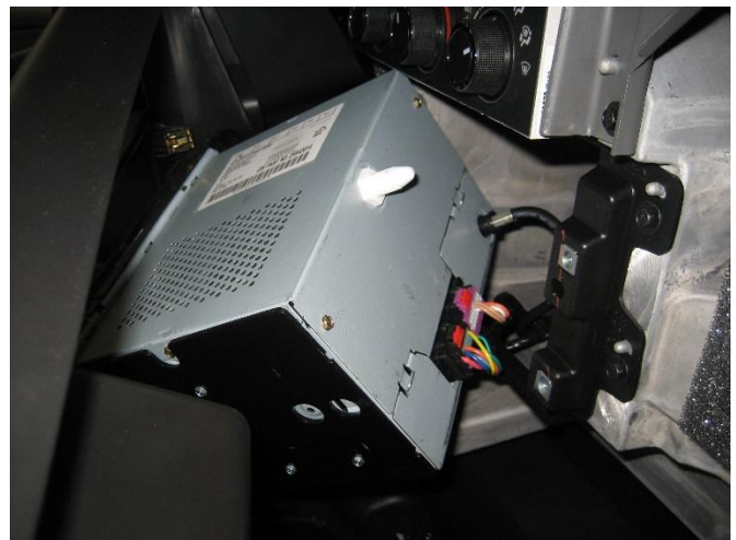
Unplug and remove radio from dash.
