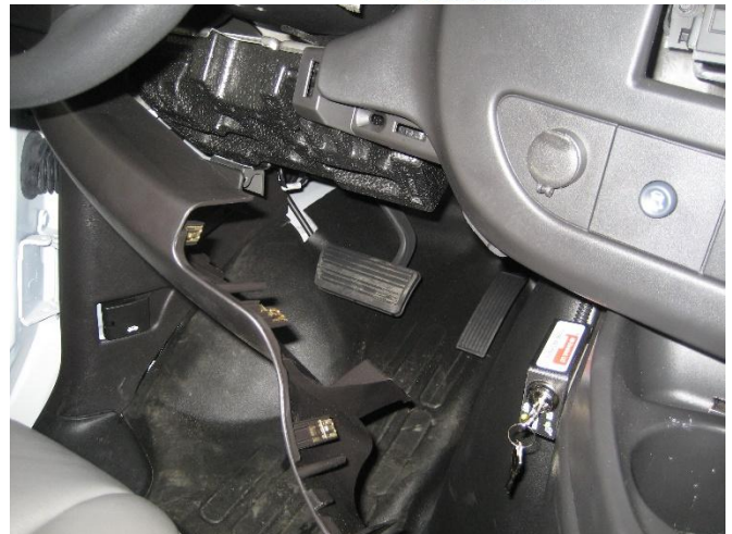
Carefully remove driver side lower dash panel. It may not be necessary to be completely removed.
