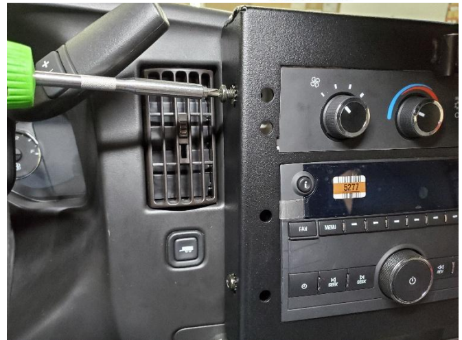
Tighten using 1/4" x 3/4" Phillips head bolts and #10 star washers.
