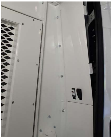
Install the middle side trim (KKM007086-PS) and wire the rear switches for rear load light, scene lights, etc.
