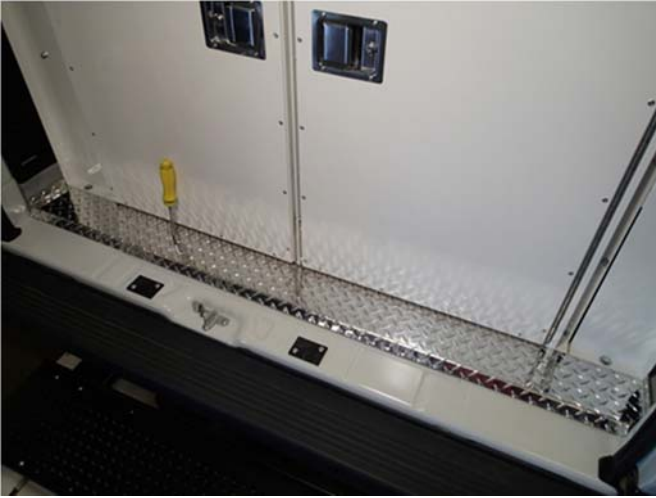
Install floor sill trim and attach with #10 x 1" (GSM33183) sheet metal screws
