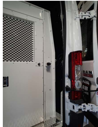
Slide the trim panel between the bulkhead and the rear Promaster door frame.
