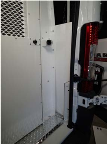
Attach trim using three (3) 1/4" x 3/4" carriage bolts and 1/4" serrated nuts.
