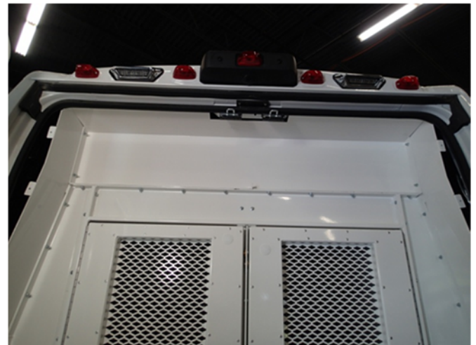
Attach Upper rear trim (KKM007096) to the top of the bulkhead frame with four (4) 1/4" x 3/4" carriage bolts and 1/4" serrated nuts.
