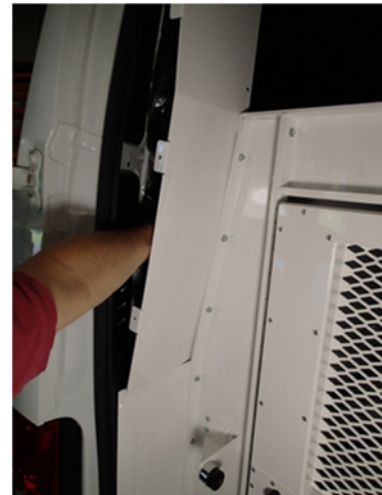
Install the middle side trim (KKM007086-DS) to the bulkhead frame using three (3) 1/4" x 3/4" carriage bolts and 1/4" serrated nuts.
