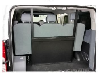
With the partition upright in the van re-install the rear seat.
