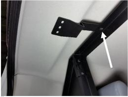
Install the upper mounting bracket to the top of the partition frame using 1/4" x 3/4" carriage bolts and nuts.
