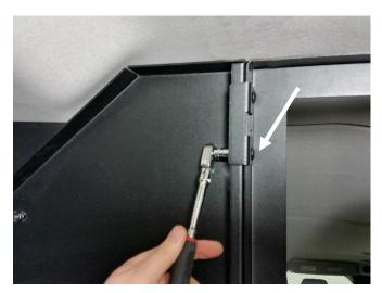
Be sure to also reattach slide bolt reinforcement brackets. Tighten hardware.
