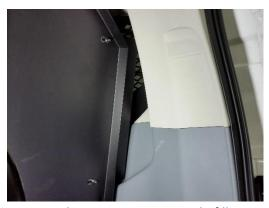
Attach passenger upper side filler panel with 1/4" x 3/4" carriage bolts and nuts. Leave a small gap between the filler and window screen to prevent noise when driving.
