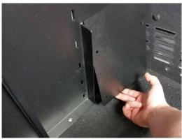
Attach passenger lower side fillers to front of partition with 1/4" x 3/4" carriage bolts and nuts.
