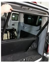
Install partition center in the van starting at the bottom.
