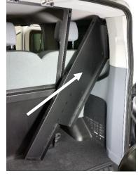
Reattach side panels to center section with 1/4" x 3/4" carriage bolts and nuts.
