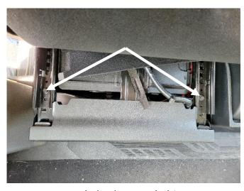
Remove rear bolts that attach driver seat to pedestal base.
