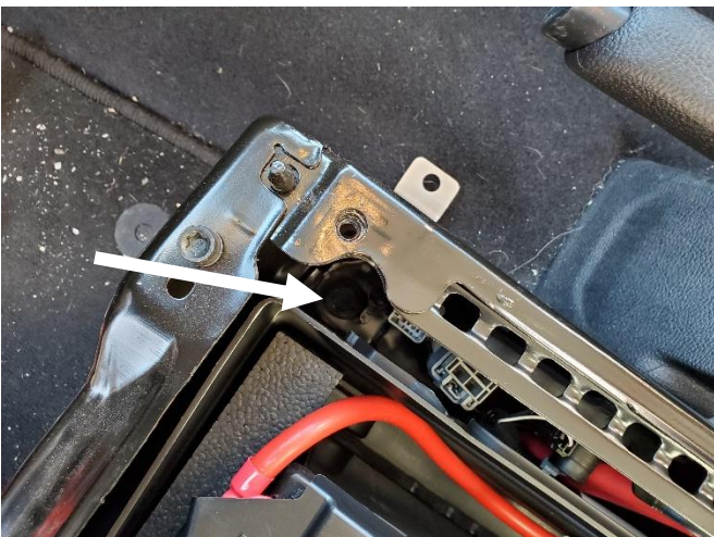
Loosen front, inner seat base bolts.
