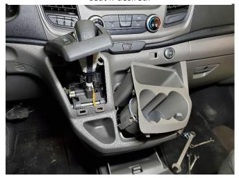
Remove cup holder assembly and shifter plate. Unplug harnesses and set panels aside.
