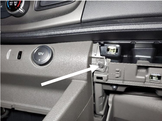
Remove OEM fastener.
