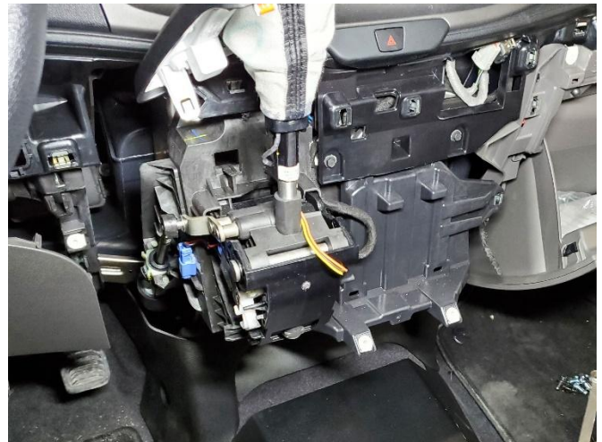
Remove OEM center dash assembly.
