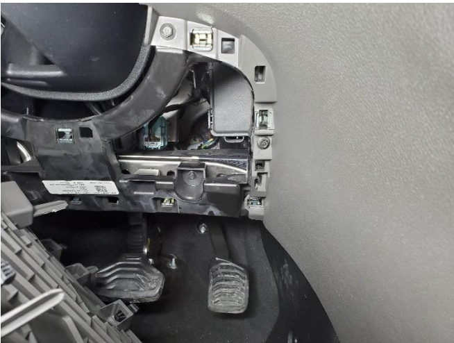
Unclip lower knee bolster trim and remove OEM fasteners from center dash assembly.
