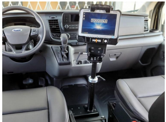
Attach pole motion device and computer. Installation is now complete.
