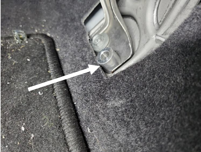
Add supplied spacer over previously removed bolt. Repeat process for other side.
