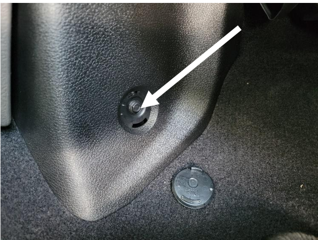
Remove covers from lower dash, trim assembly. Remove hardware and trim.
