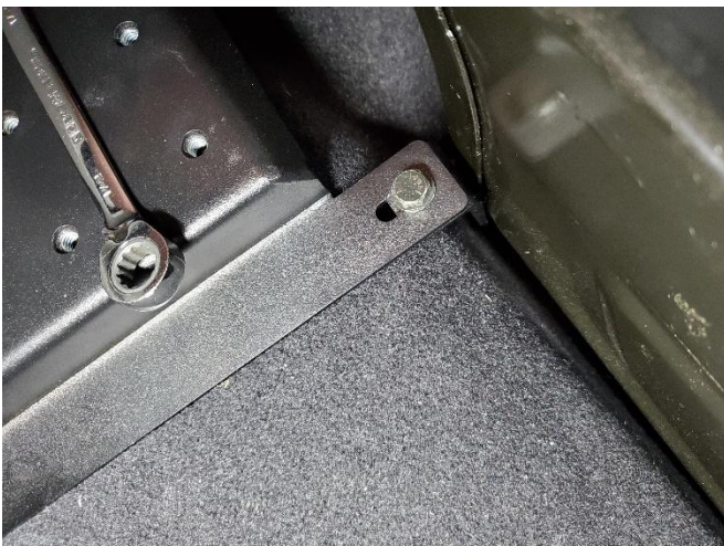
Attach HDM base to rear-mounting brackets using 5/16" x 3/4" bolts, split lock washers and flat washers.
