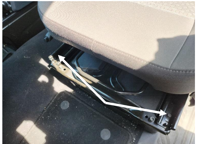
Remove front bolts that attach driver seat to pedestal base.
