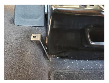
Place driver side rear-mounting bracket under seat base and tighten bolt. Reinstall previously removed driver seat.
