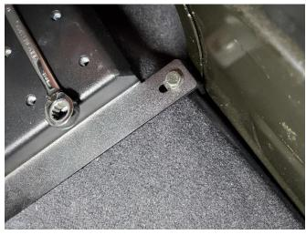
Attach HDM base to rear-mounting brackets using 5/16" x 3/4" bolts, split lock washers and flat washers.
