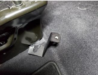
Place passenger side rear-mounting bracket under seat base and tighten bolt. Reinstall previously removed passenger seat.
