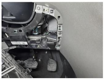
Unclip lower knee bolster trim and remove OEM fasteners from center dash assembly.
