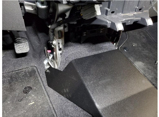
Slide HDM base up to lower dash brace and align with spacers.
