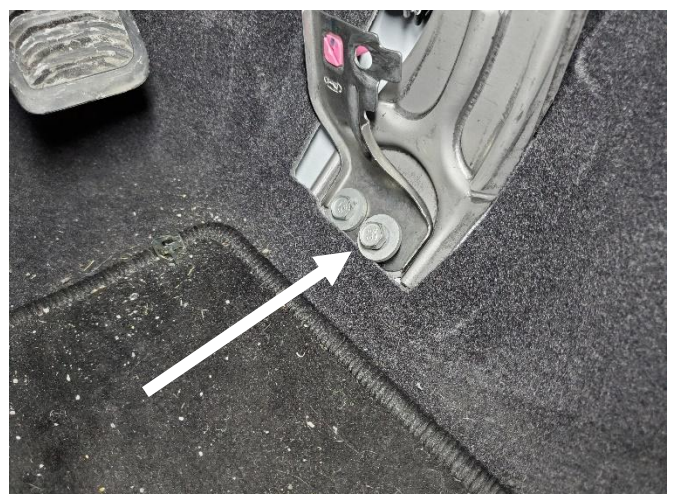
Remove rear bolt from lower dash brace on each side. Hardware will not be reused.
