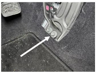
Remove rear bolt from lower dash brace on each side. Hardware will not be reused.
