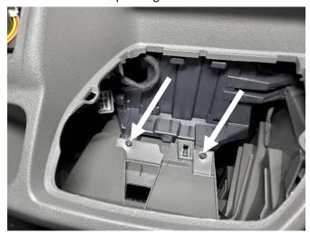
Remove OEM fasteners from lower trim assembly.
