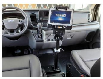
Attach pole motion device and computer. Installation is now complete.
