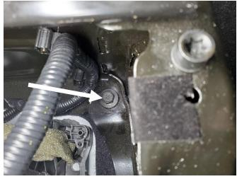
Remove inner front seat base bolt on passenger side. This can be accessed without removing the seat if desired.
