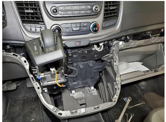
Remove trim assembly from center, dash.
