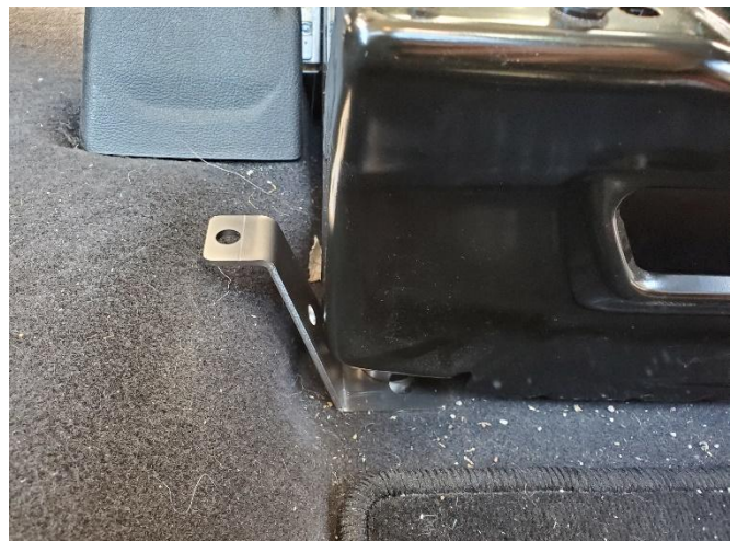
Place driver side rear-mounting bracket under seat base and tighten bolt. Reinstall previously removed driver seat.
