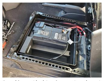
Lean driver seat back to gain access to under seat battery tray.
