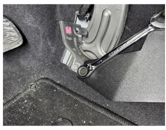
Tighten hardware. Reinstall all previously removed dash trim.
