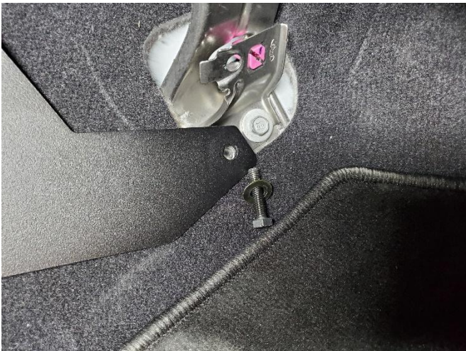
Attach base to floor with supplied M8 x 35mm bolts, split lock washers and flat washers.
