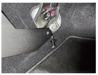
Attach base to floor with supplied M8 x 35mm bolts, split lock washers and flat washers.
