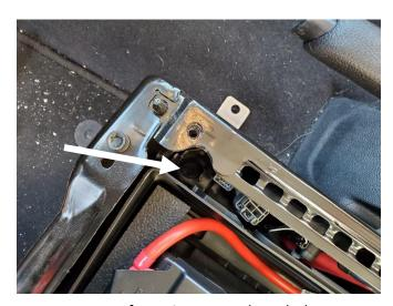
Loosen front, inner seat base bolts.
