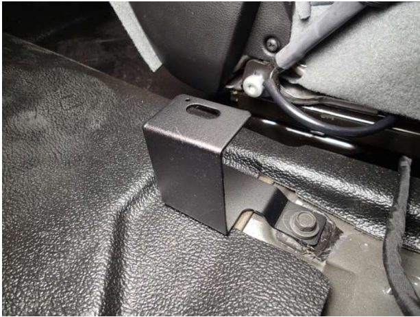
Optional CM006057 Driver side rear bracket with GSM33745 (M8 x 35mm bolt) and GSM31007 (3/8 flat washer) (included in C-B66 kit)
