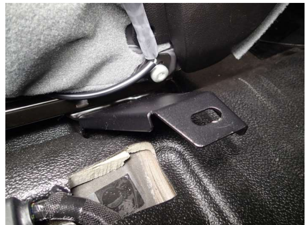
Optional CM006059 Passenger side rear bracket with GSM33001 (1/4 x 3/4 screws) and GSM31005 (1/4 flat washers) (included in C-B66 kit)
