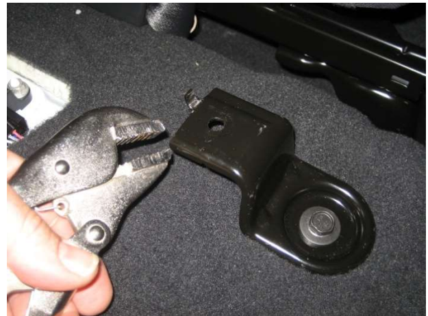
Make sure you leave the OEM center seat brackets in place. Small tabs on driver side brackets will have to be bent down. OEM driver side forward bracket shown.
