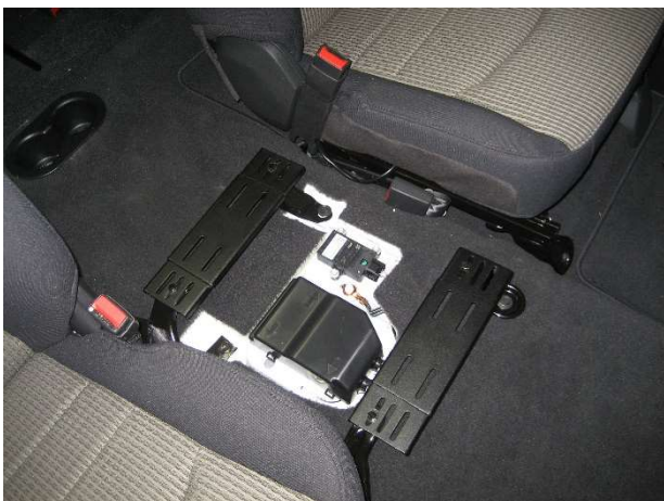
Attach hump bracket center plates onto the seat brackets with \frac{1}{4} " x \frac{3}{4} " hex head bolts, fender washers, lock washers and nuts.
