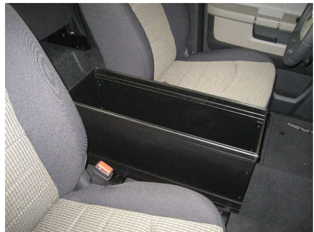
Determine position of the console housing and attach to the center plates with \frac{1}{4} " x \frac{3}{4} " hex head bolts and nuts provided.
