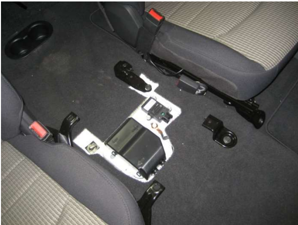
Remove OEM center seat pad section. This shows the standard 2013 Dodge OEM seat brackets. Older trucks have slightly different brackets, but mounting works the same.
