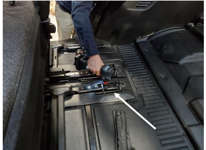
Flip seat seats forward to access hardware.
