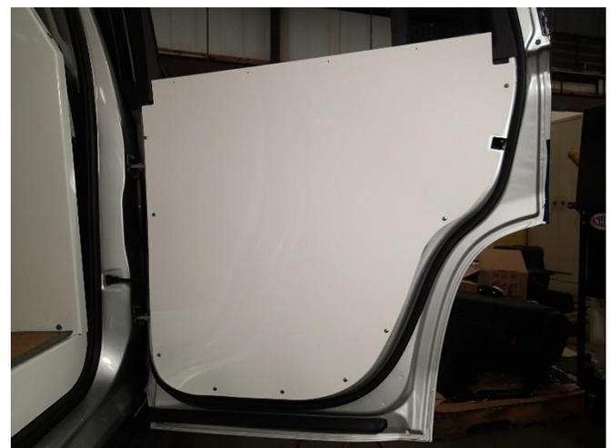
Hook top of door panel into rubber window gasket.
