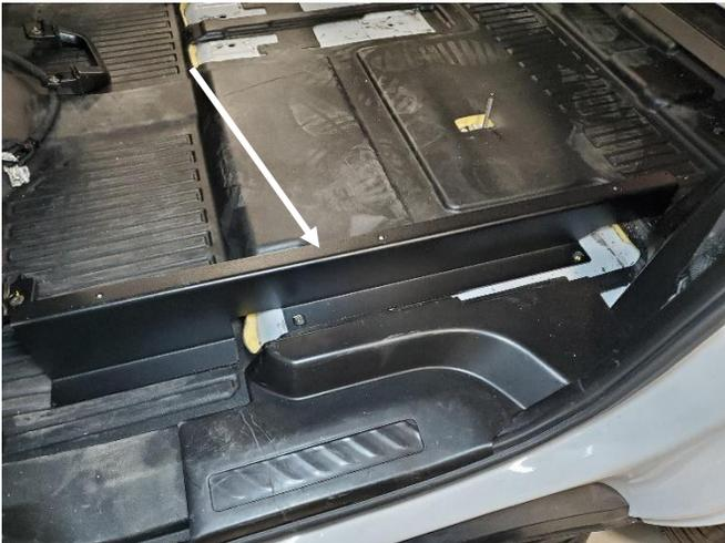
Using previously removed seat mounting hardware, attach driver side floor mounting bracket.
