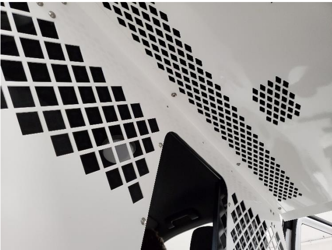
Attach ceiling to bulkheads with 1/4" x 3/4" Phillips head bolts and flat washers.
