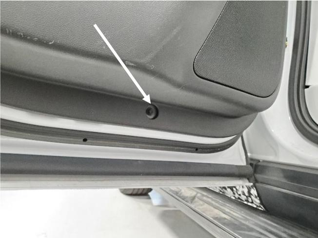
Remove screw at bottom of door panel.
