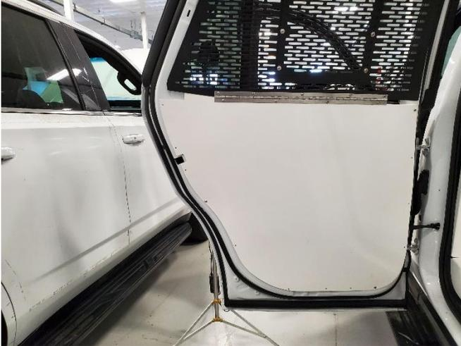
Align the hinge mounting holes to holes in the door panel. Attach hinge with # 10 x 1/2 Phillips pan head sheet metal screws.
