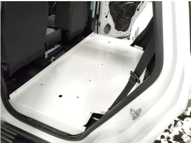
Attach stiffener (angle) bracket to bottom of K9 floor with (3) 1/4" x 3/4" Phillips head bolts and flat washers. Place floor in vehicle and properly line up to brackets.
