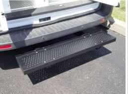
Tighten all hardware and check to make sure the step is even and level.
