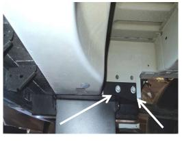
Remove the two bolts shown in the picture and install the Main bracket using the four (4) removed factory bolts.
