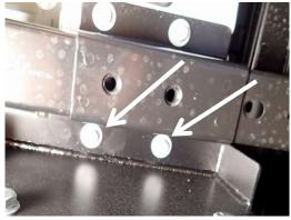
On the driver side remove the two bolts located on the inside of the rear frame rail. Keep bolts for reinstall in the next step.
