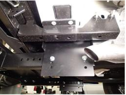
Determine the height you want to set the rear step and insert two (2) 1/2"x 1.5" bolts, (4) 1/2" washers, and (2) nylock nuts.
