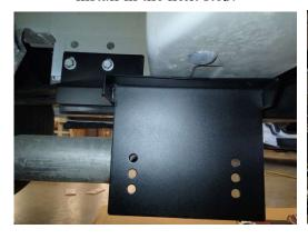
Repeat the mounting procedure for the driver side bracket
