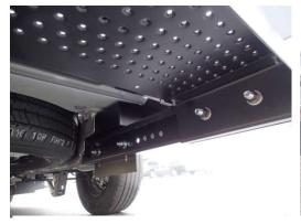
Loosen the eight (8) 1/4" nylock nuts from the step assembly and slide the step onto the previously install channel supports using four (4) 1/2"x 3.5" bolts, (8) 1/2" washers and four (4) 1/2" nylock nuts.
