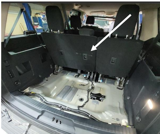
Remove third row seats if applicable. Note: Tape over unused seat mount holes in floor.
