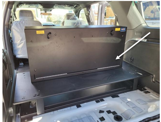
Attach C-SBX-101 to mount plate with 1/4" x 3/4" Hex head bolts, lock washers, flat washers and serrated nuts.
