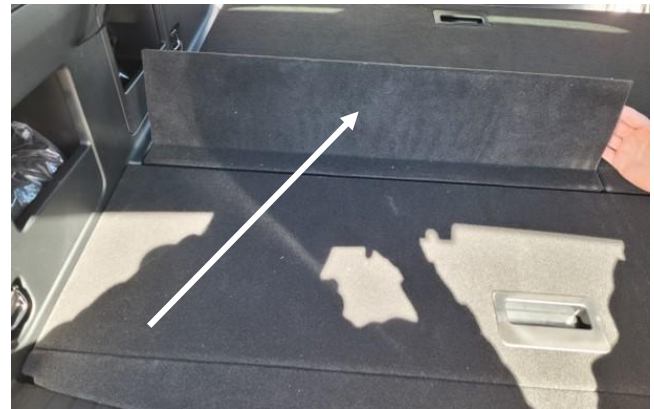
Prior to re-installing OEM rear storage bin, the hinged flaps must be cut off in order to fit.
