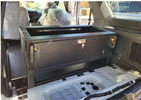
Attach SBX-1000 series drawer to mount plate with 5/16" x 3/4" Hex head thread-forming screws.
