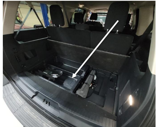
Remove OEM rear storage bin / compartment.
