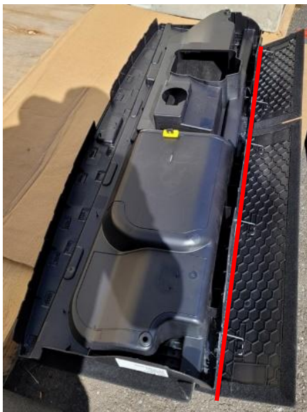
Detach springs from OEM rear storage bin flaps and cut flaps approximately at hinge point shown by the red line. Reinstall rear storage bin.
