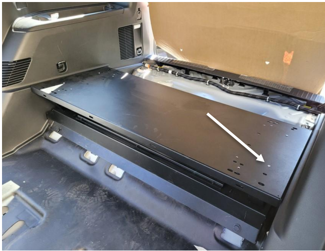
Attach mount plate to risers with 10-32 X 1/2 Phillips flat head machine screws and nuts.
