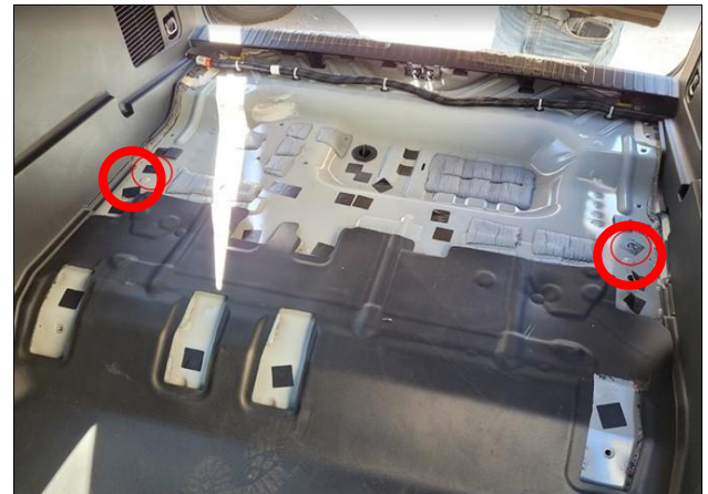
For a vehicle with no third row seat, remove tape over two circled holes and tap with M12x1.75 thread.
