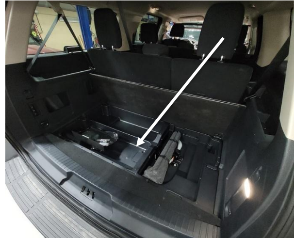
Remove OEM rear storage bin / compartment.
