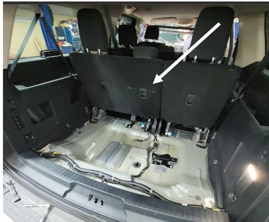
Remove third row seats if applicable. Note: Tape over unused seat mount holes in floor.
