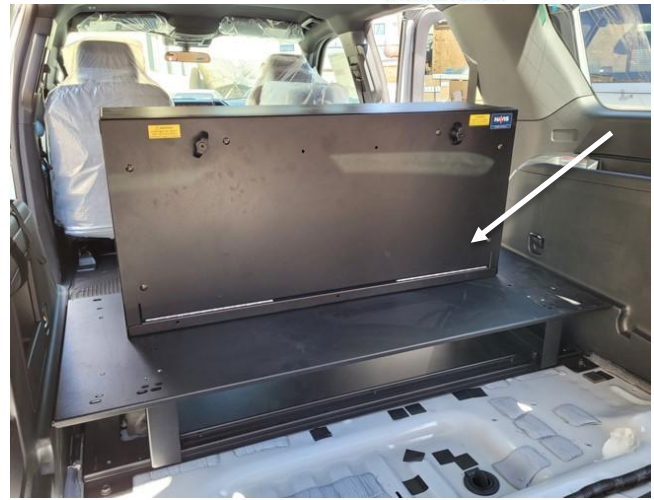
Attach C-SBX-101 to mount plate with 1/4" x 3/4" Hex head bolts, lock washers, flat washers and serrated nuts.
