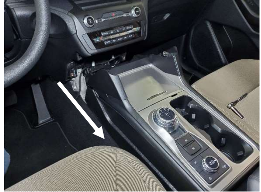
Slide OEM console away from dash and remove from vehicle.
