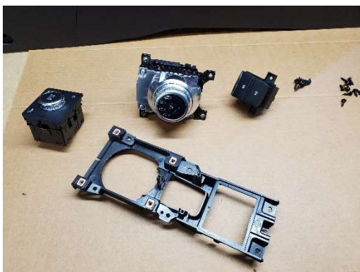
Unscrew the shifter and emergency brake switch from the bezel.
