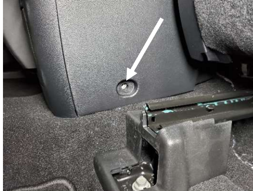
Remove (1) bolt each side at rear of OEM console. (10mm socket)
