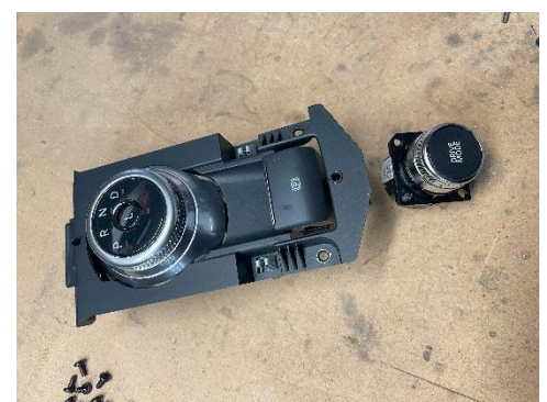
Unscrew the drive mode switch, parking brake and shifter from the bezel.
