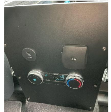
Relocate OEM 12v sockets and rear HVAC control to new end panel. Attach control with supplied 10-32 x 1/2" screws and flat washers.
