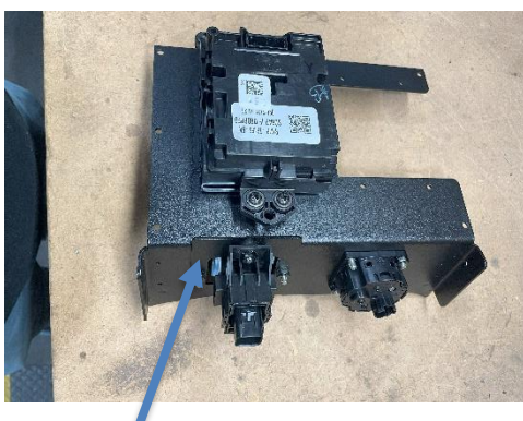
Install 42552 backing plate using supplied 8-32 keps nuts
