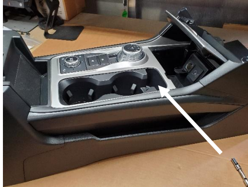
Gently pry up top of console using a panel removal tool.
