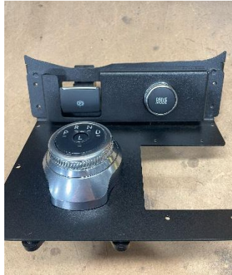
Install previously removed parts into new shifter plate using supplied 8-32 x 1/2" Phillips machine screws and flat washers.
