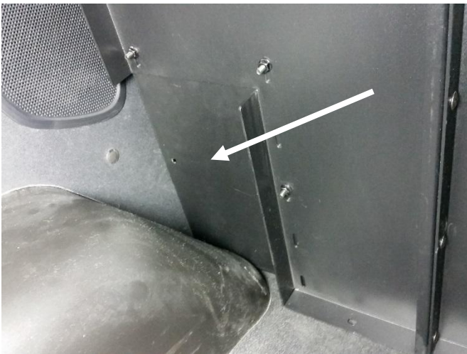
Attach lower side fillers to front of partition with 1/4" x 3/4" carriage bolts and nuts.
