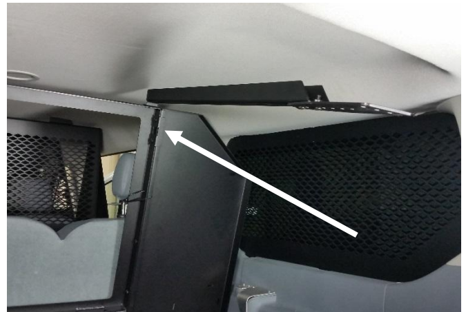
Reattach side panels to center section with 1/4" x 3/4" carriage bolts and nuts. Be sure to also reattach slide bolt reinforcement brackets.
