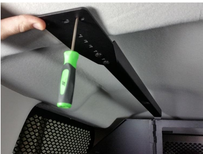
Verify sheet metal above headliner once bracket is lined up using a straight pick tool.
