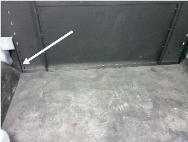
Determine lower placement of the partition in relation to the wheel wells
