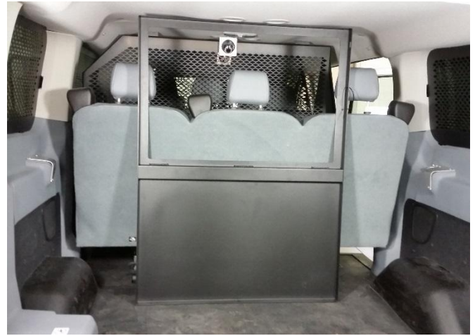
Install center of partition into the van.
