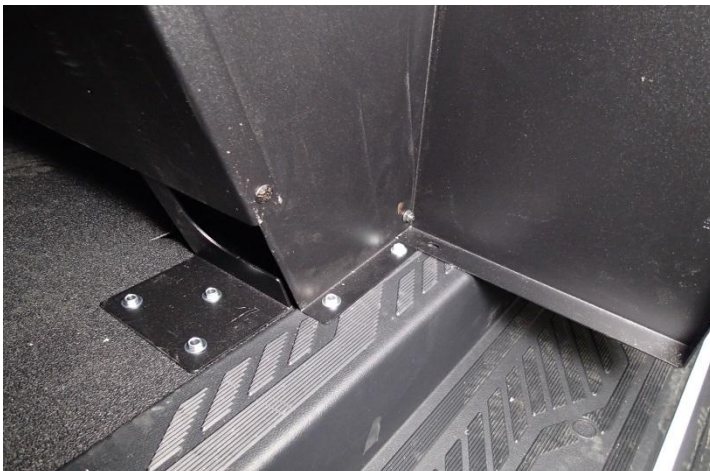
Attach passenger side bracket and side panel to floor with five (5) 1/4 x 1" Lag screws. Take caution not to strip the holes.
