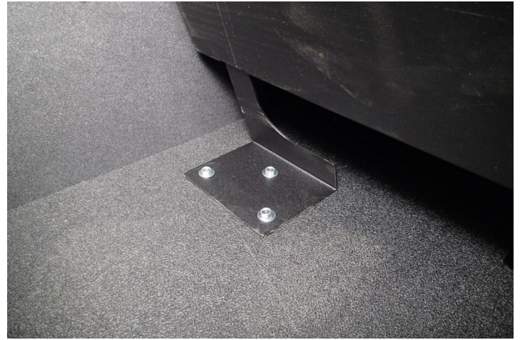
Attach driver side bracket to floor with three (3) 1/4 x 1" Lag screws. Take caution not to strip the holes.
