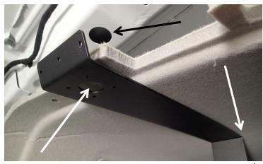
Hold upper mount bracket to the mid-forward headliner (2<sup>nd</sup> section from front) and align large hole to large hole in the roof rib. Mark the headliner where the forward part of bracket will come through and cut a slot in the headliner.
