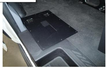
Mount block off plate (HS-PA007323) to floor. Carefully drill floor with 1/8 bit and attach with twelve (12) #10 x 1.25" screws (GSM34157)
