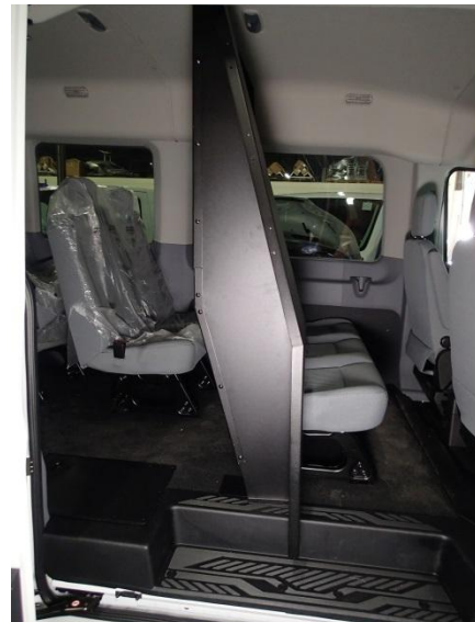
Attach driver side upper and lower side filler panels using five (5) 1/4 x 3/4" carriage bolts and serrated nuts. Filler panels angle toward front of vehicle
