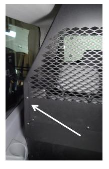
Attach the side reinforcement bracket to the upper and lower base using four (4) 1/4 x 3/4" carriage bolts and nuts.
