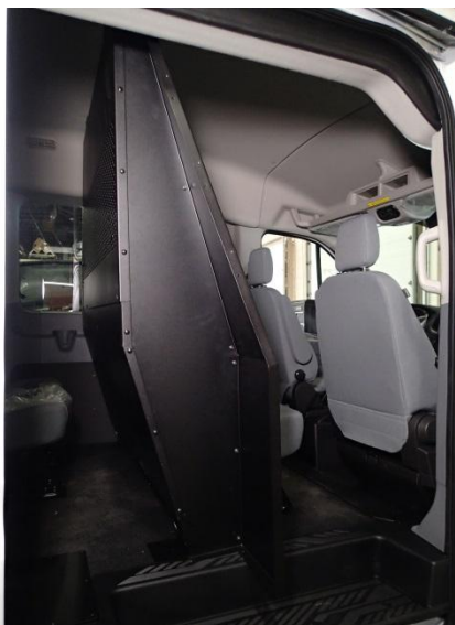
Attach passenger side bracket and side panel to floor with five (5) 1/4 x 1" Lag screws. Take caution not to strip the holes.
