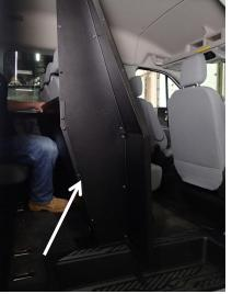
While holding the upper main panel in place lean both main panels back and install 1/4 x 1/2" carriage bolts into the holes. Have another person attach the nuts from the forward side.
