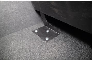
Attach driver side bracket to floor with three (3) 1/4 x 1" Lag screws.
