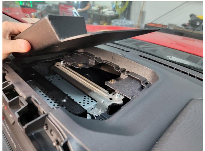
Place upper mounting tray onto dash.
