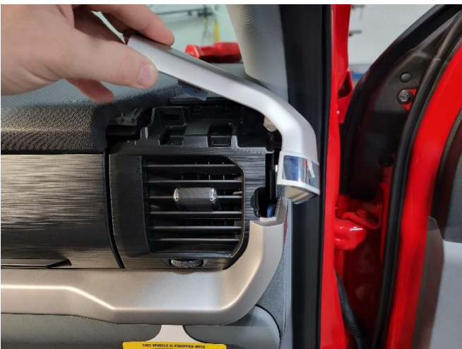
Unsnap trim around passenger vent assembly.
