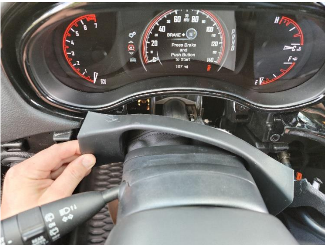
Remove trim around lower instrument cluster.
