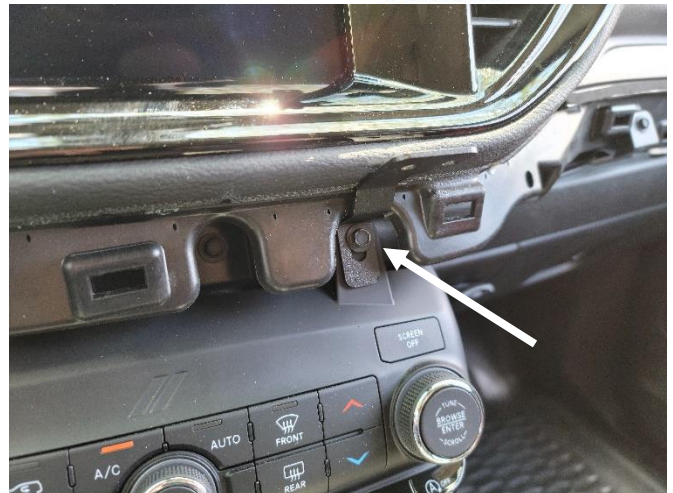
Install lower mounting tab using previously removed OEM fastener.
