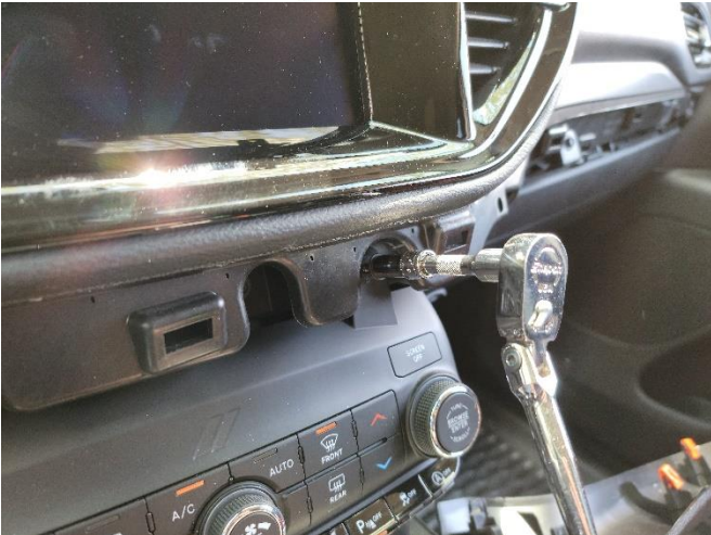
Remove 7mm head fastener from lower trim.
