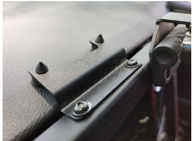
Ensure upper bumper bracket is snug against dash.
