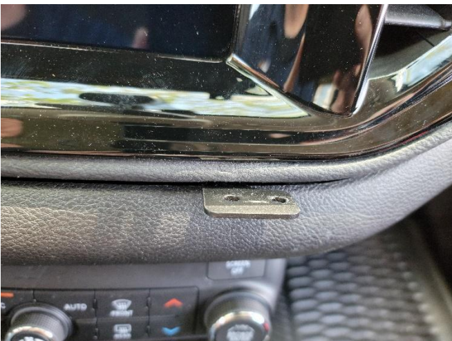
Ensure lower mounting tab is level when sticking out of dash.
