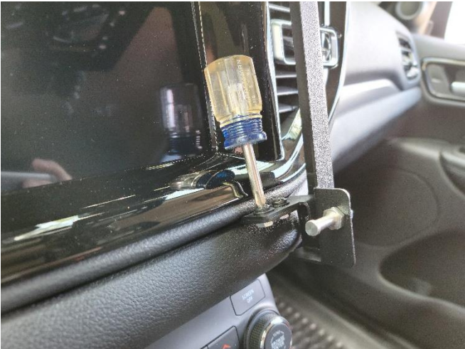
Attach lower frame using supplied #10 screws, washers, and keps nuts
