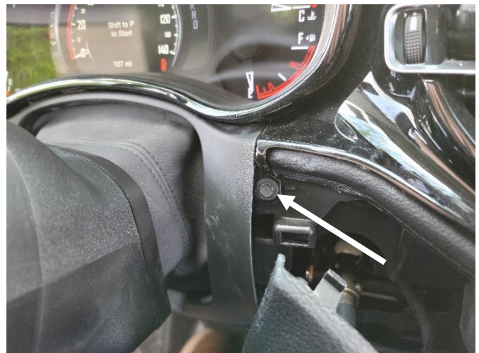
Remove 7mm head fastener from center trim.
