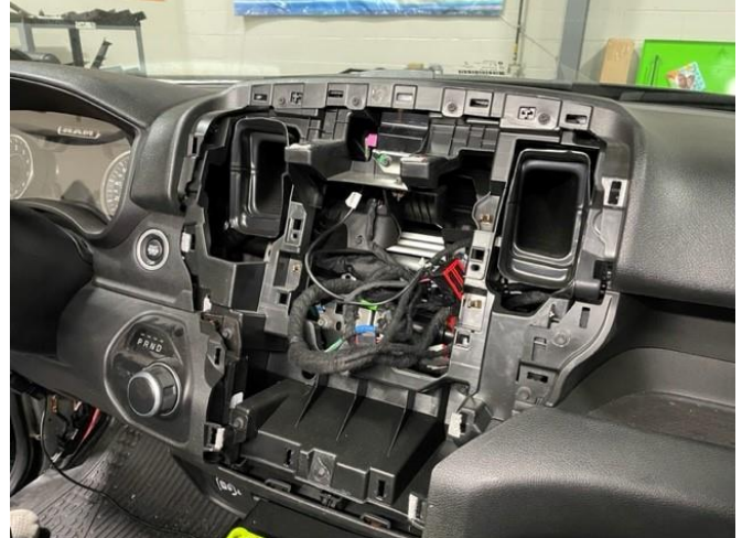
Carefully remove center instrument panel.
