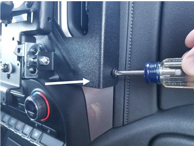
Loosely start the hardware for the side mounting bracket. Tighten the hardware while pressing the frame against the dash.
