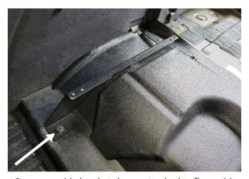
Passenger side bracket shown attached to floor with M10 x 1.5 x 45mm hex bolt.
