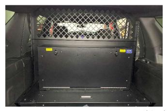
Attach angle bracket to SBX box under door hinge with 1/4" x 3/4" bolts, washers and nuts. Attach SBX box to floor box with 1/4 x 3/4 bolts and star washers Attach lid with 1/4" x 5/8" Button head screws.
