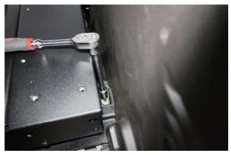
Tighten floor bracket hardware. Attach side top trim brackets with  $1/4" \times 3/4"$  Hex bolts and star washers. Place optional C-SBX-101 box on floor mount box.
