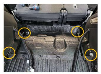
Determine 3rd row seat bolt locations in forward floor and loosely attach long front brackets with supplied M10 bolts.
