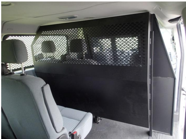
Completed P-MID-2 Middle Partition installation
