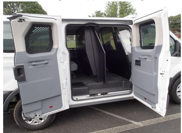
Completed P-MID-2 Middle Partition installation
