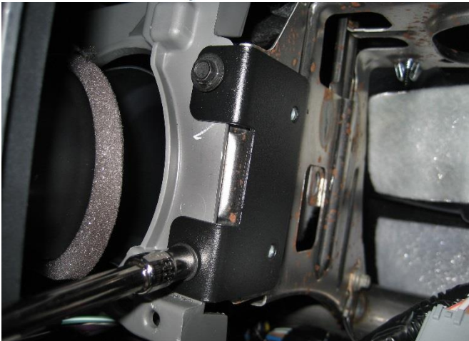
Using OEM radio screws, attach driver and passenger side CM002987 support brackets. Driver side shown.
