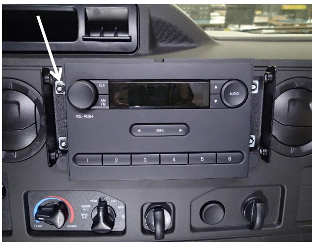
Plug in radio wiring and slide radio back into the dash. Attach radio onto the four (4) bracket studs with 8/32 nuts.
