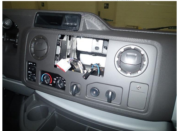
Reconnect plugs and reinstall center dash panel.
