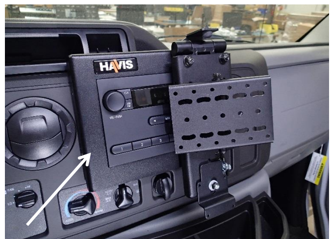
Place frame and hinge mount assembly onto support brackets.
