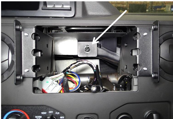
Insert and loosely attach CM009573 Main support bracket to forward dash frame with 3/8" x 1" Hex Bolt, (2) flat washers and Nylock nut.
