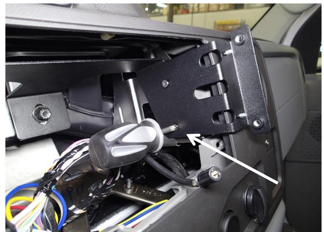
Line up main bracket side holes with the side bracket threaded holes. Attach with 10-32 x 5/16" flat head screws. Two (2) each side.
