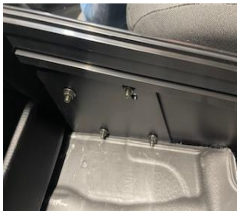
VS-1110-DUR: Attach the front of the console to the front mounting bracket with (8) 1/4" x 3/4" carriage bolts and (8) serrated.
