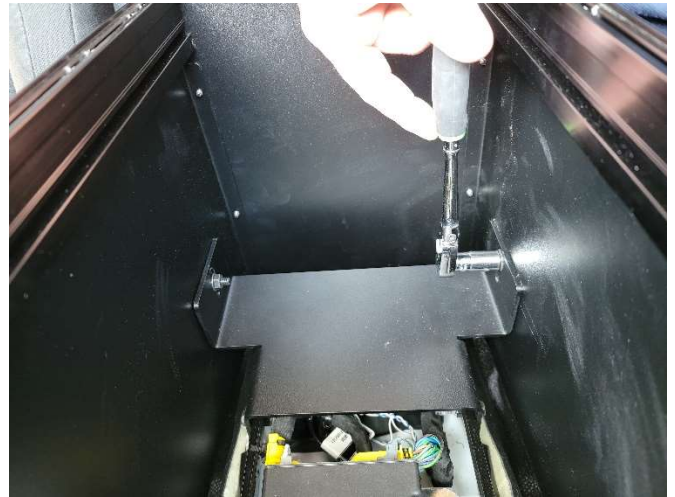
Attach rear of console to rear mounting bracket with (2) \frac{1}{4} " x \frac{3}{4} " carriage bolts and (2) serrated nuts.
