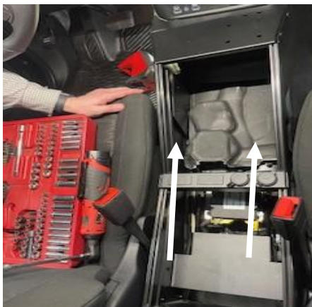
Place console over the mounting brackets and slide towards the dash.
