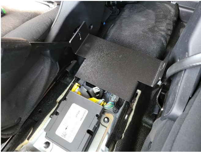
Position the rear mounting bracket over the rear mounting tab as shown.
