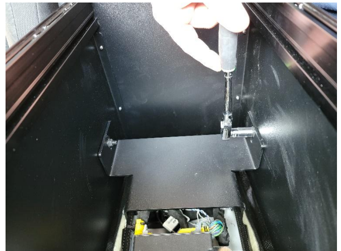
Attach rear of console to rear mounting bracket with (2) 1/4" x 3/4" carriage bolts and (2) serrated nuts.
