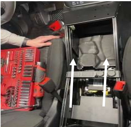
Place console over the mounting brackets and slide towards the dash.
