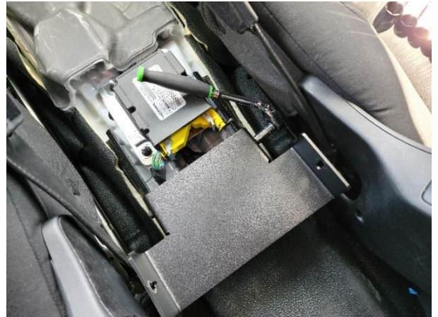
Loosely attach the rear mounting bracket using a 10mm socket and the OEM bolts.
