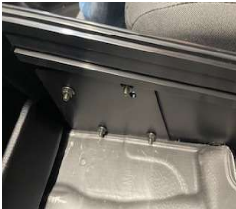
VS-1110-DUR: Attach the front of the console to the front mounting bracket with (8) \frac{1}{4} " x \frac{3}{4} " carriage bolts and (8) serrated.
