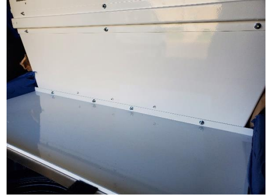
Place rear cargo filler onto rear mounting brackets and line up to rear wall of kit. Attach to rear wall of kit using (4) 1/4" x 3/4" carriage bolts and serrated nuts.
