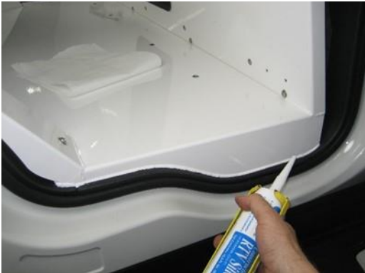
Neatly silicone / caulk the lower seams to shed water out of vehicle.
