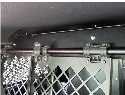
Confirm smooth slide and lock function on front egress door.
