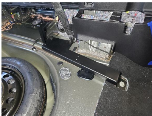
Attach rear floor side mounting brackets in rear of vehicle using holes and hardware from third row seat.
