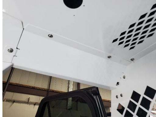
Attach upper trim panel with 1/4" x 3/4" Phillips head bolts and flat washers. Forward hole through front bulkhead uses a 1/4" x 3/4" carriage bolt and nut.
