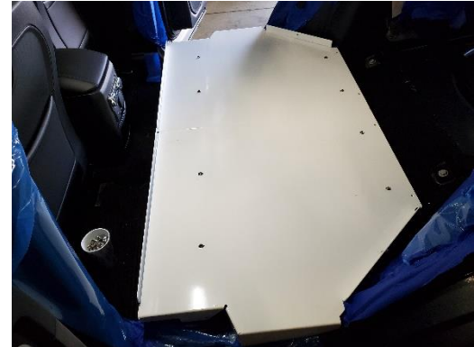
Place floor into vehicle and loosely attach to front and middle floor brackets with 1/4" x 3/4" Phillips head bolts and flat washers.
