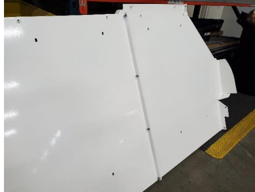
Before the floor is installed, both sides must be bolted together. Use (4) 1/4" x 3/4" carriage bolts and serrated nuts.
