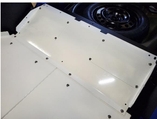
Place rear angled floor section into vehicle. Attach to forward floor and rear bracket with 1/4" x 3/4" Phillips head bolts and flat washers.
