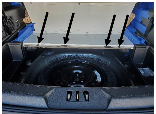
Add Velcro circles to rear cargo floor adaptor "L" bracket.
