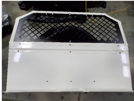
Attach screen and brace with 1/4" x 3/4" carriage bolts and serrated nuts. Smooth carriage bolt heads go on dog side of bulkhead.
