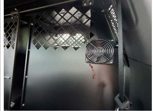
Example mounting location for the optional air circulation fan. # K9-A-102
