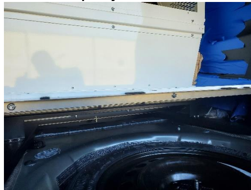
Attach rear cargo floor adaptor bracket to rear cargo filler plate using (3) 1/4" x 3/4" Phillips head bolts, flat washers and serrated nuts.
