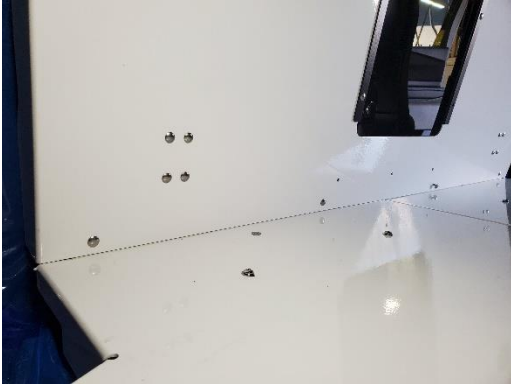
Attach bulkhead to floor using (4) 1/4" x 3/4" carriage bolts and serrated nuts.
