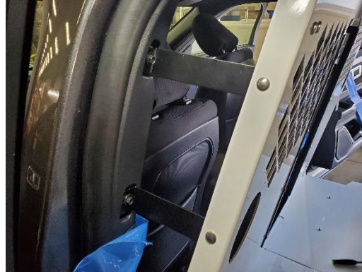
Loosely attach front bulkhead to "B" pillar brackets with 1/4" x 1/2" carriage bolts and serrated flange nuts. Bracket goes on inside of bulkhead flange.
