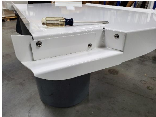
Attach cover plate with supplied hardware.
