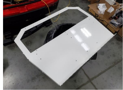
Carefully lay rear bulkhead on flat work surface prior to installation.
