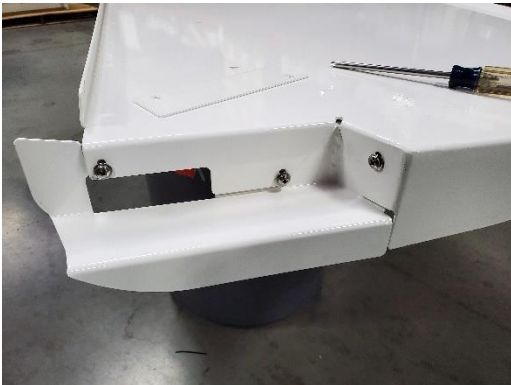
Attach with (3) 1/4" x 3/4" Phillips head bolts and flat washers.
