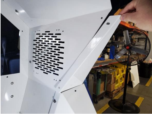
Attach upper rear trim panel to rear side wall and lower trim panel with 1/4" x 3/4" pan head Phillips bolts and flat washers.
