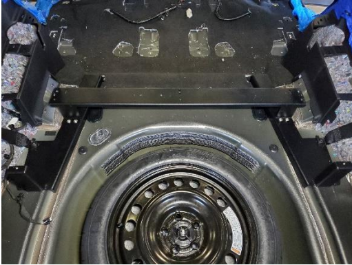
Attach rear cross support to both rear floor brackets using (4) 1/4" x 3/4" Phillips head bolts and flat washers.
