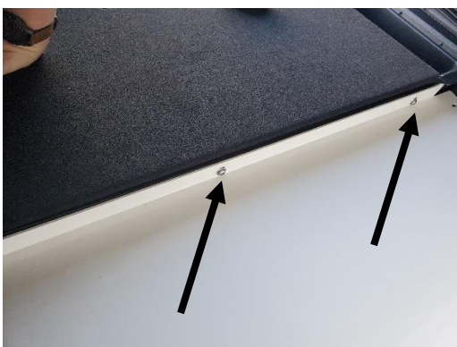
Place rear OEM floor in vehicle and line up to bracket. Press to secure to Velcro circles.
