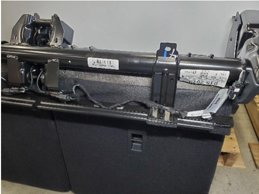
Remove harness from seats. Plug harness in to plug on driver side of cargo area. Plug seat belts back in.
