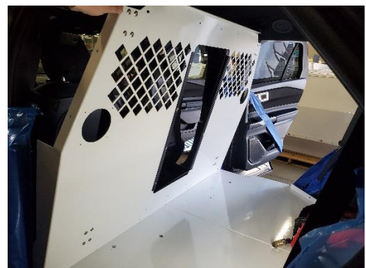
With the help of a second person, carefully place front bulkhead into vehicle.
