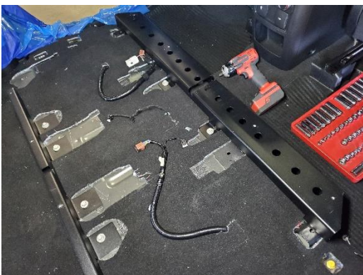
Use OEM seat bolts to attach K9 kit front floor bracket to OEM seat mount locations.
