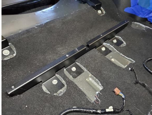
Attach rear floor bracket using previously removed seat bolts.
