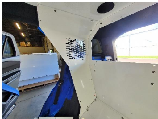
Attach rear side wall into kit with 1/4" x 3/4" Phillips head bolts and flat washers.
