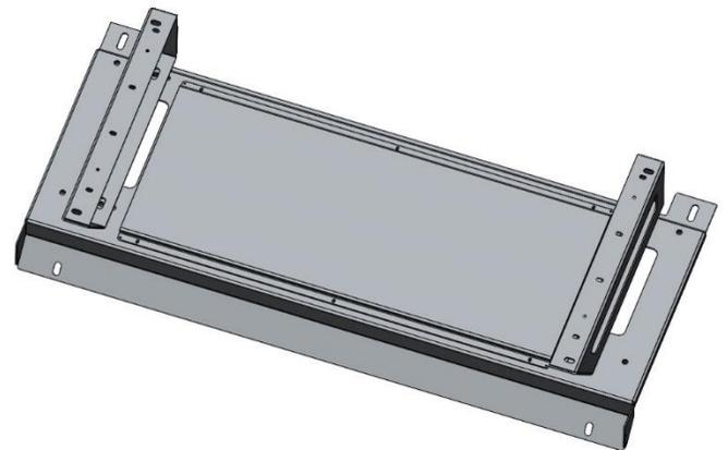
Attach riser brackets to base with 5/16" X 3/4" Hex head bolts, lock washers and flat washers.
