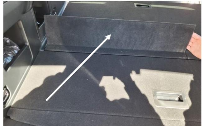
Prior to re-installing OEM rear storage bin, the hinged flaps must be cut off in order to fit.
