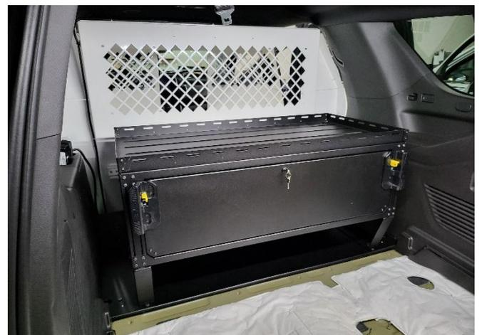
Attach the rear trim to the bottom of the SBX-1000 drawer using #10 sheet metal screws into pilot holes drilled in step 1.
