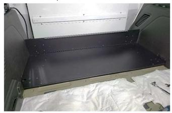
Attach the trim panel to the rear flange of the base plate using the supplied  $1/4-20 \times 1/2$ " flathead bolts.
