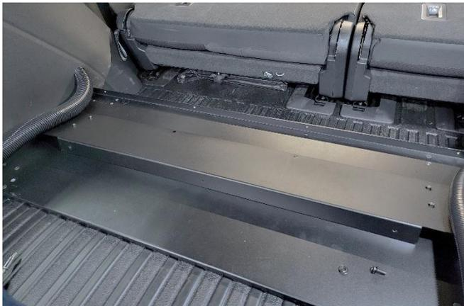
Carefully place the trim panel against the rear flange of the SBX-5008 or SBX-5010 base plate. Angling the trim piece as shown in photo can help with trim clearance as it is positioned.
