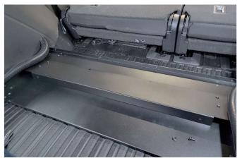
Carefully place the trim panel against the rear flange of the SBX-5008 or SBX-5010 base plate.
