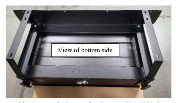
Preassemble risers and trim panel to bottom SBX-1000 drawer in stack. If desired, at this time use trim measurements from previous page to mark and drill three 1/8" pilot holes for #10 sheet metal screws to be attached later.
