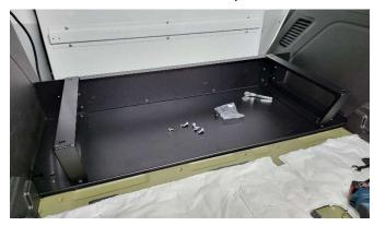
Attach the risers to the trim panel using supplied 1/4" x 3/4" Phillips head bolts, washers, and lock washers and to the base plate using supplied 5/16" x 1" hex bolts, washers, and lock washers. Attach drawer to the risers with 5/16 thread forming bolts.
