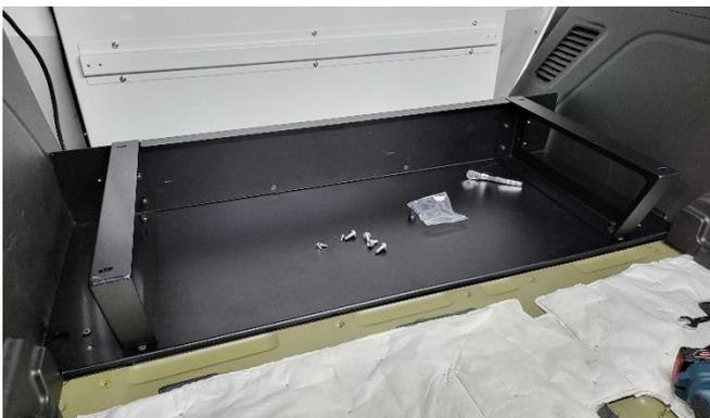
Attach the risers to the trim panel using supplied 1/4" x 3/4" Phillips head bolts, washers, and lock washers and to the base plate using supplied 5/16" x 1" hex bolts, washers, and lock washers. Attach drawer to the risers with 5/16 thread forming bolts.
