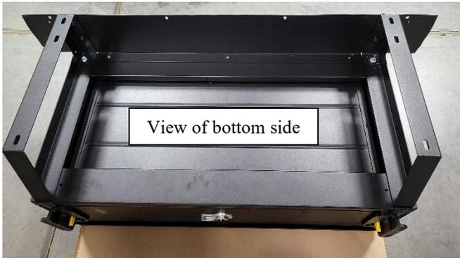
Preassemble risers and trim panel to bottom SBX-1000 drawer in stack. If desired, at this time use trim measurements from previous page to mark and drill three 1/8" pilot holes for #10 sheet metal screws to be attached later.
