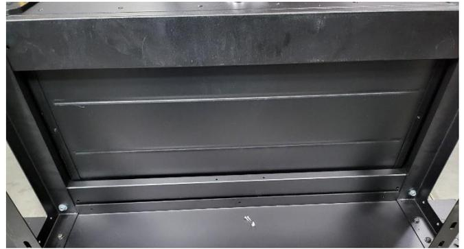
Run the screws into the pilot holes to form the threads while there is easier access to the holes. If parts were preassembled, remove the trim panel after this is complete. Risers can remain attached.
