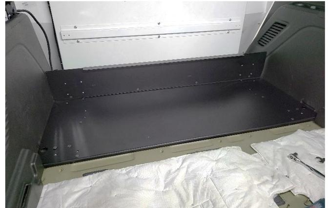
Attach the trim panel to the rear flange of the base plate using the supplied 1/4"-20 x 1/2" flathead bolts.
