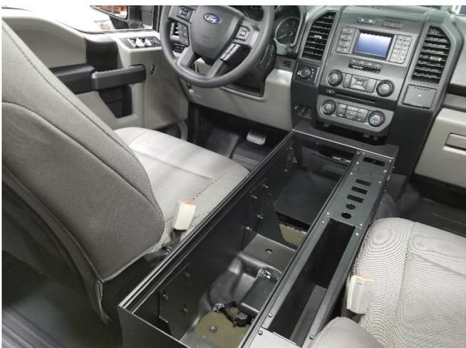
Place console with floor mount brackets into the vehicle.
