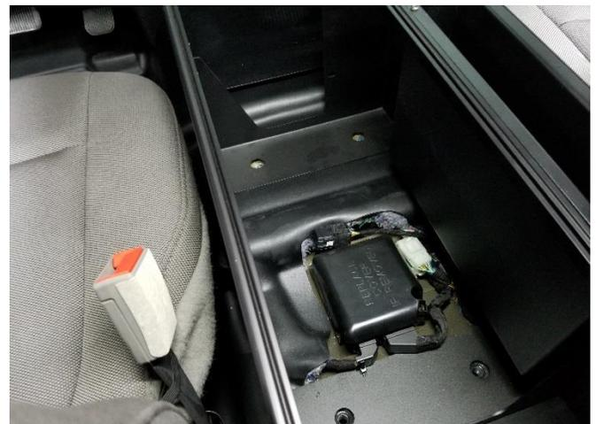
Slide console forward until the mounting brackets line up with the OEM mounting points in floor.
