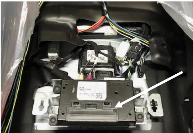
**NOTE:** Some vehicles include an OEM SmartLink / Telematics module mounted to transmission hump using the same bolts needed for the rear console bracket.
