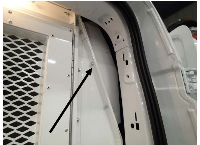
Remove three previously installed 1/4" carriage bolts and slide upper filler panel between the kit and the side of the van. Install with the three previously removed carriage bolts.
