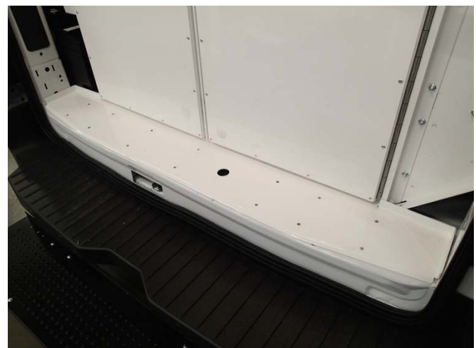
Line up rear door sill (KKM006910) to the rear bulkhead.
