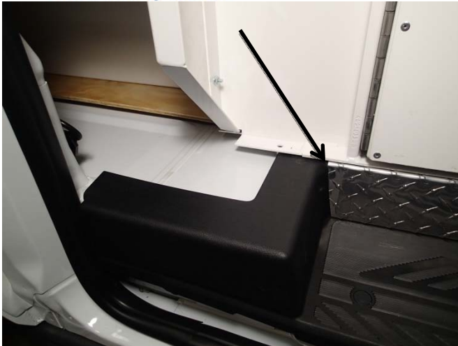
Angled side of the trim piece should contour the factory step trim
