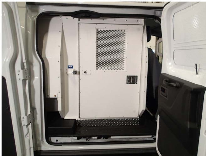
Completed side door and floor trim installation.
