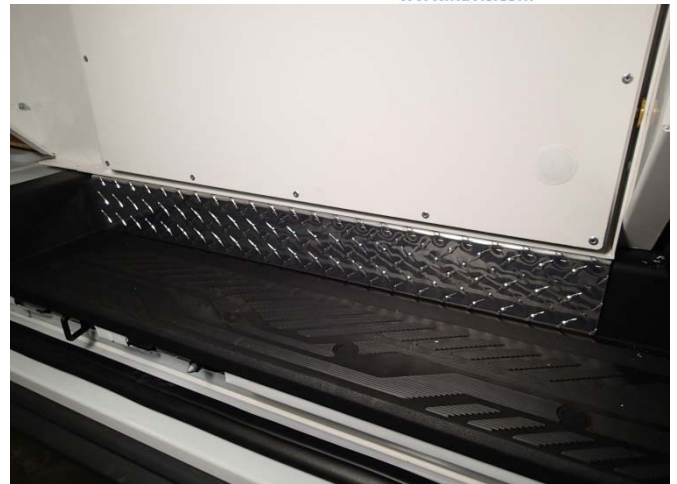
Make sure trim is even and continue with door frame installation using #10 x 1" Phillips pan head screws for door frame and trim.
