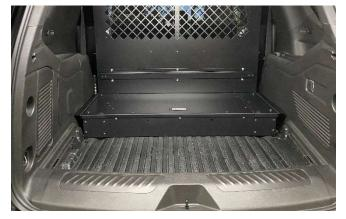
Attach lid with 1/4" x 5/8" Button head screws Installation complete.
