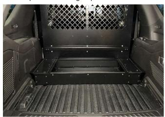
Place main box assembly onto brackets and attach with (10) 1/4" x 3/4" Hex bolts and star washers. Mount equipment onto removable tray as desired.
