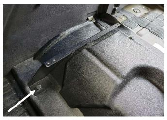
Passenger side bracket shown attached to floor with  $M10 \times 1.5 \times 45 mm$  hex bolt.
