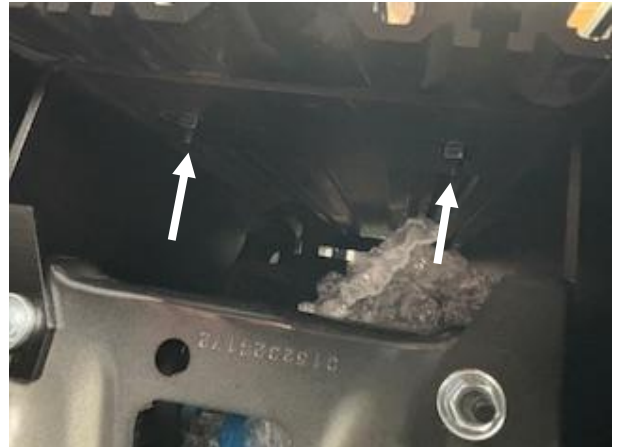
Slide (2x) ¼-20 x ¾ hex screws in both sides of extrusion and at both ends (4 screws total) and attach to mounting brackets with ¼-20 hex serrated flange nuts
