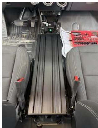
Fully tighten all hardware. Tunnel mount is shown after installation is complete.
