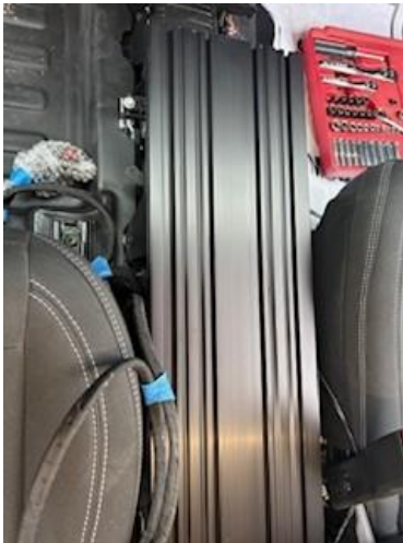
Place 28" extrusion on mounting brackets.
