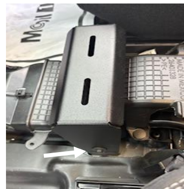
Attach front mounting bracket using OEM hardware
