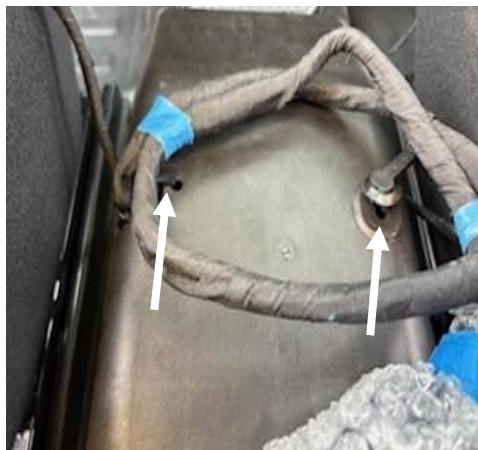
Remove both wire management components from OEM cover plate
