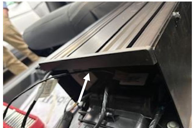
Attach trak mount gasket and end cap to both ends of extrusion
