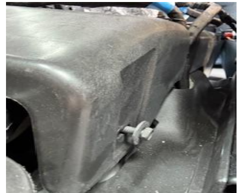
Remove hardware from OEM cover plate using 10MM socket
