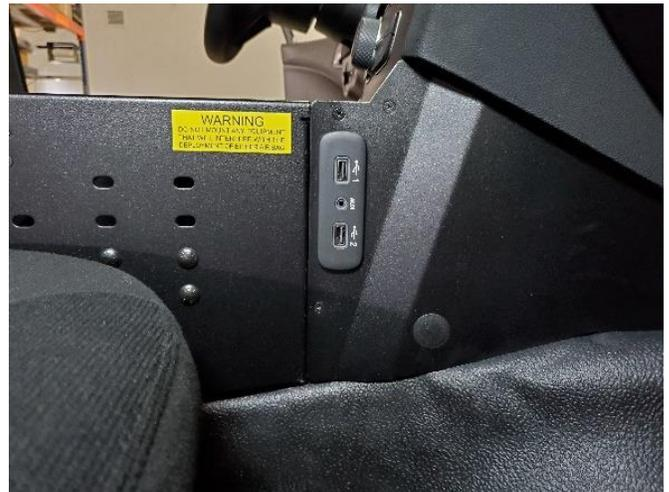
After connecting the aux panel wiring, snap panel into side trim panel.
