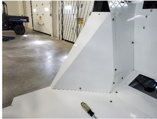
Attach K9 lower filler into kit using 1/4" x 3/4" pan head Phillips bolts and flat washers.
