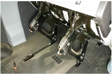
When both latches are released push the seat forward to remove. The front is hooked and will need to be slid rearwards.
