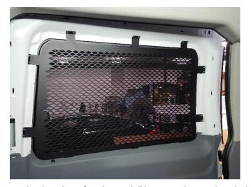
Determine location of each guard. Place guard up to the window frame, mark and pre drill mount holes with a 1/8" drill bit. (Slight bending of the tabs may be necessary to ensure a proper fit)
