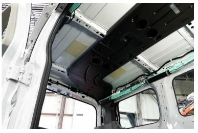
Removing the headliner is recommended but not required. Removing the headliner will be required if installing a Front or Middle Partition.
