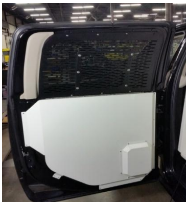
With upper mount bracket attached to window guard, mark mounting hole locations on upper door/window frame. Drill 5/32" holes and attach with # 10 x 1/2" flat head sheet metal screws
