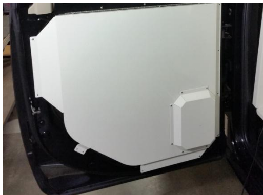
Install door panel using #10 x 1/2" Phillips pan head sheet metal screws.
