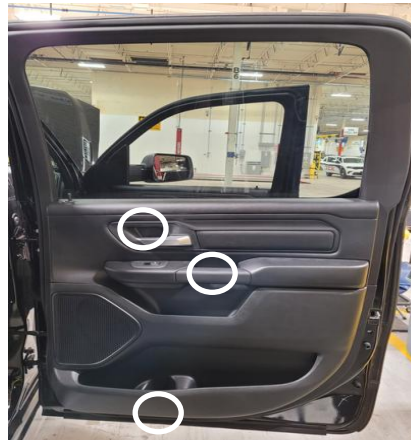
Remove door panels first by removing push clips around perimeter of door panel.
