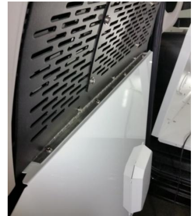
Align the hinge mounting holes to holes in the door panel. Attach hinge with # 10 x 1/2" Phillips pan head sheet metal screws.
