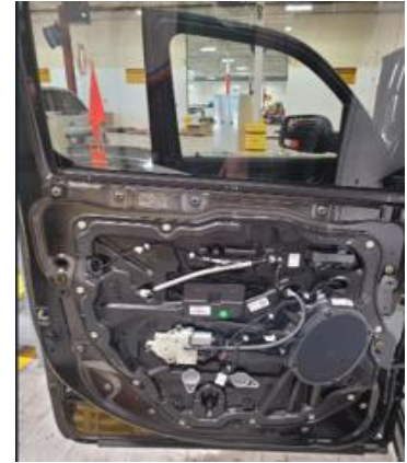
Remove bolts behind access cover behind inner door handle
