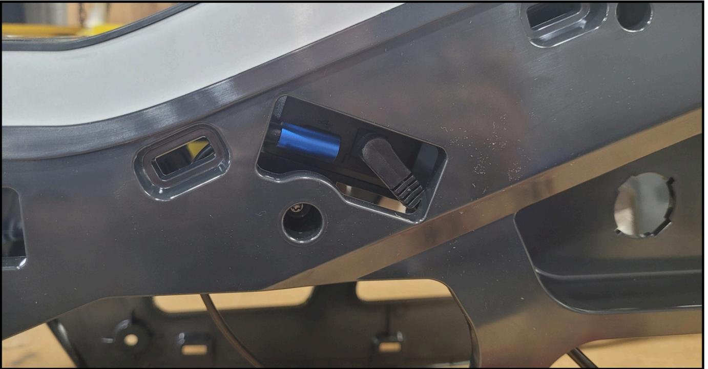
To attach the printer, screw QTY. 2 of M2.6 Phillips head screws (17805) through two holes in the bin and then into the printer. Do not overtighten screws – printer threads can strip.
