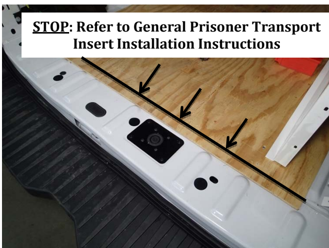
Overall length of plywood should be at least 102" long (for 100" insert) or 122" long (for 120" insert) to match insert length plus rear sill trim. Additional piece needed for side entry area. Cut 4x4" square spacers and install in corners as shown. These prevent the wood from bowing when the kit is bolted down later.
