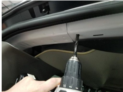
Remove partition and upper plastic trim panel. Drill upper pilot holes in metal frame out to 25/64"
