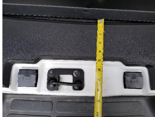
Make sure the floor is level and even. It should be 8.5" from door opening.
