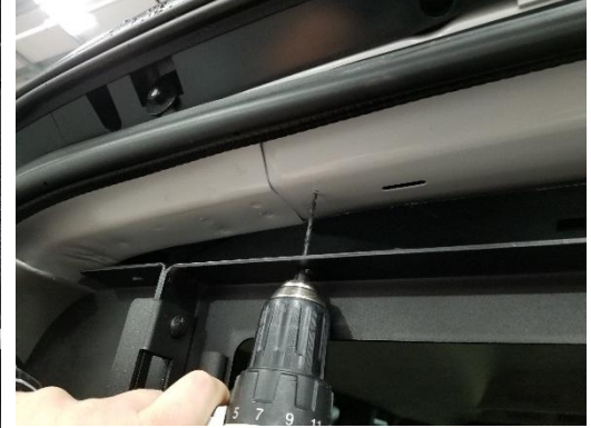
Pre-drill two (2) 1/8" pilot holes in top trim and metal cross support. Use holes in partition frame to determine drill location. Upper trim panel has been removed to show detail.
