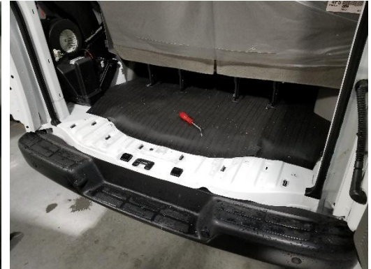
Remove lower plastic sill plate and drill lower holes out to 25/64"
