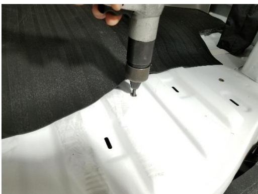
Install 1/4" rivnuts into the holes and tighten using a rivnut gun or rivnut tool.
