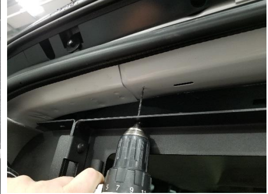
Pre-drill two (2) 1/8" pilot holes in top trim and metal cross support. Use holes in partition frame to determine drill location.
